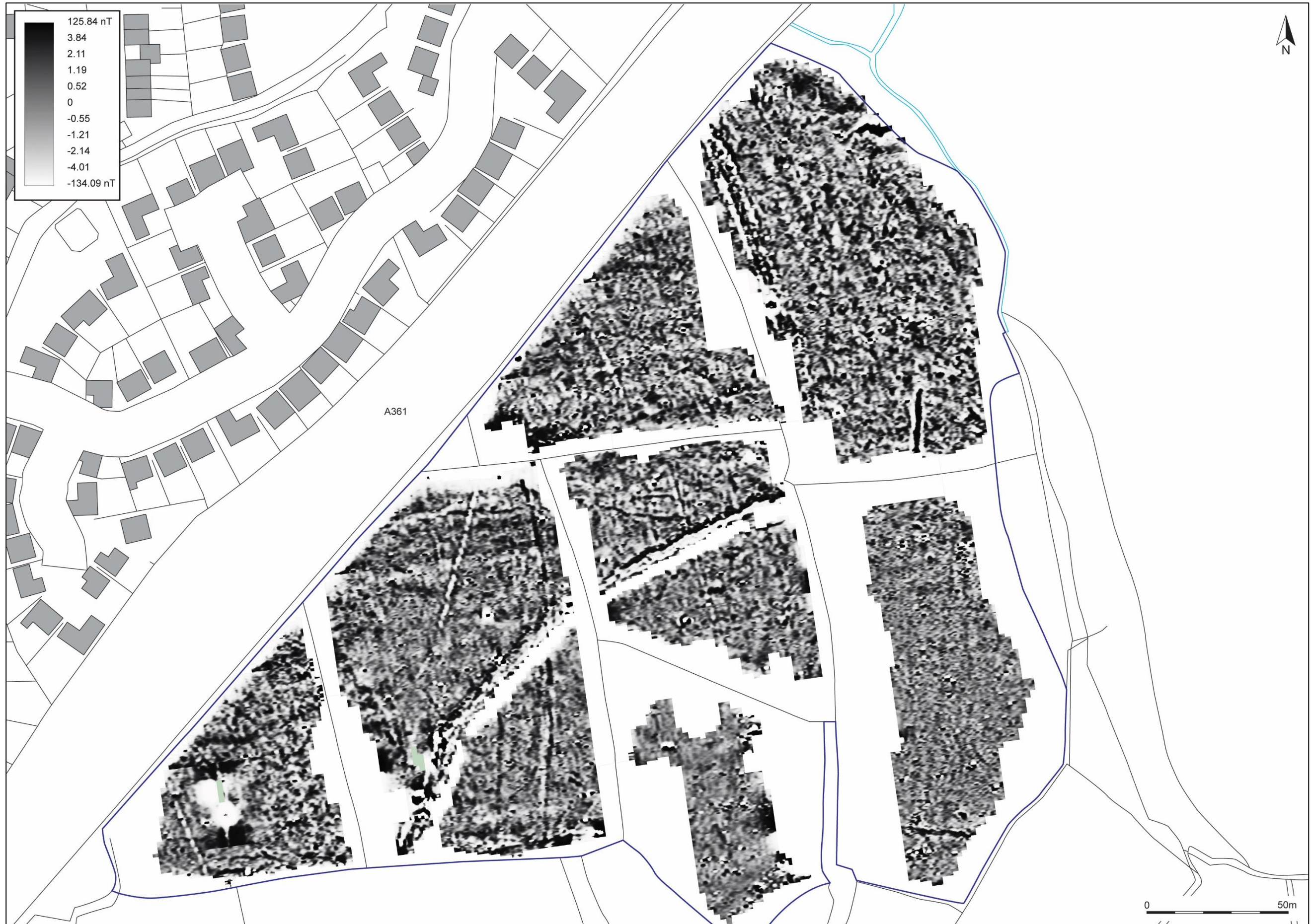
FIGURE 3: SHADE PLOT OF GRADIOMETER SURVEY DATA; BANDWEIGHT EQUALISED, GRADIATED SHADING.
