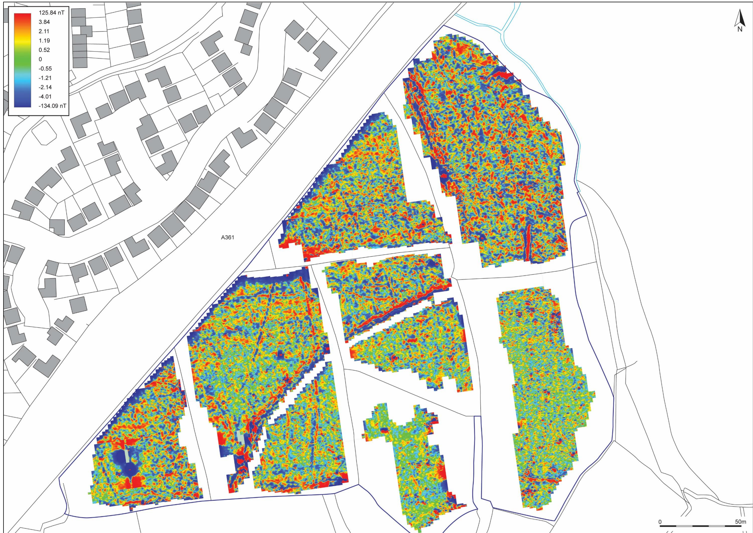
RED-BLUE-GREEN SHADE PLOT OF GRADIOMETER SURVEY DATA; BAND WEIGHT EQUALISED, GRADIATED SHADING.
