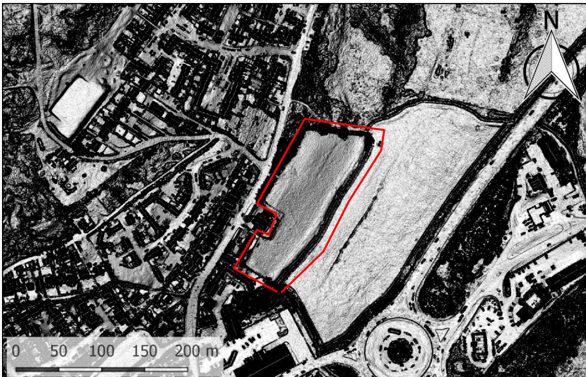
FIGURE 7: IMAGE DERIVED FROM 50CM DSM LIDAR DATA, SHOWING THE SITE (INDICATED)(PROCESSED USING QGIS VER2.18.2, TERRAIN ANALYSIS/SLOPE, VERTICAL EXAGGERATION 3.0). DATA: © ENVIRONMENT AGENCY COPYRIGHT AND DATABASE RIGHTS 2017; CONTAINS OS DATA © CROWN COPYRIGHT AND DATABASE RIGHTS 2017.
