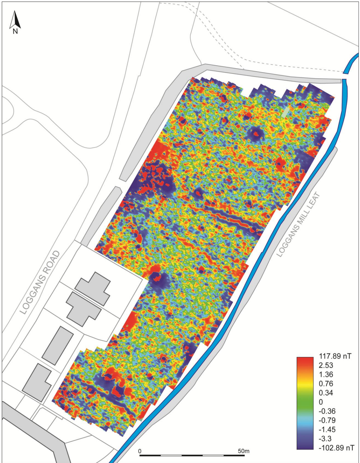
RED-BLUE-GREEN SHADE PLOT OF GRADIOMETER SURVEY DATA; BAND WIEGHT EQUALISED; GRADIATED SHADING.
