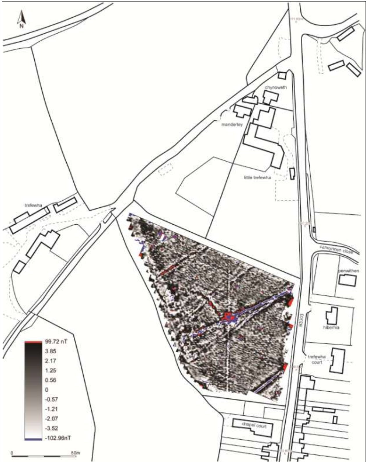
FIGURE 14: RED-GREY-BLUE SHADE PLOT OF GRADIOMETER SURVEY DATA: GRADIATED SHADING; BAND WEIGHT EQUALISED.
