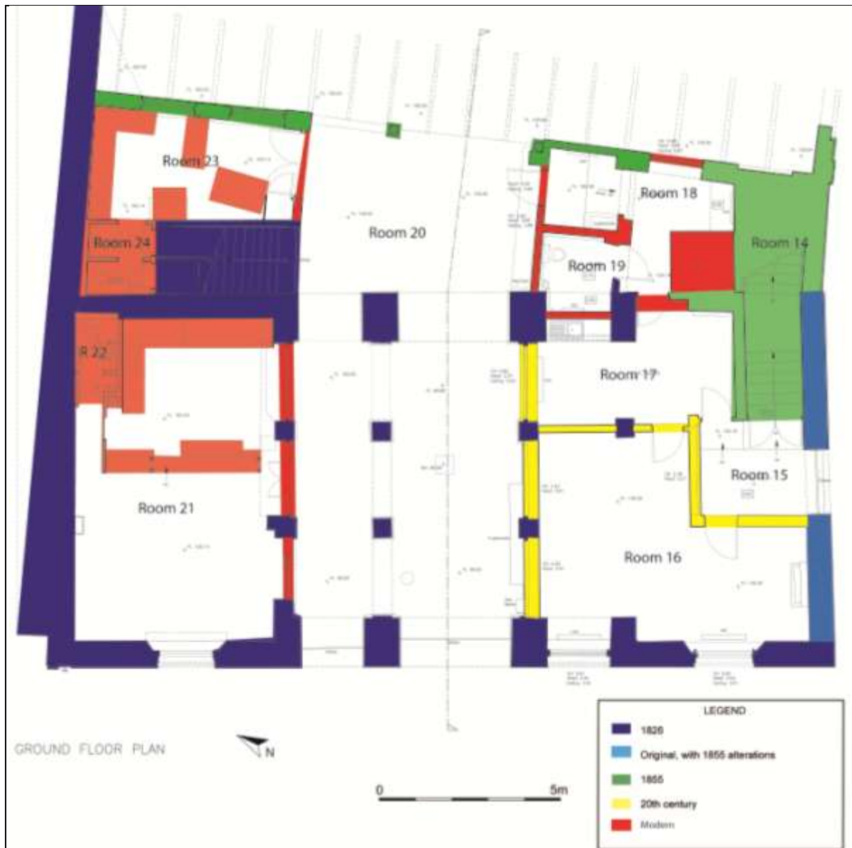
FIGURE 2: PHASE PLAN OF THE GROUND FLOOR.
