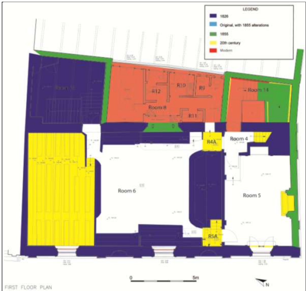
FIGURE 3: PHASE PLAN OF THE FIRST FLOOR.
