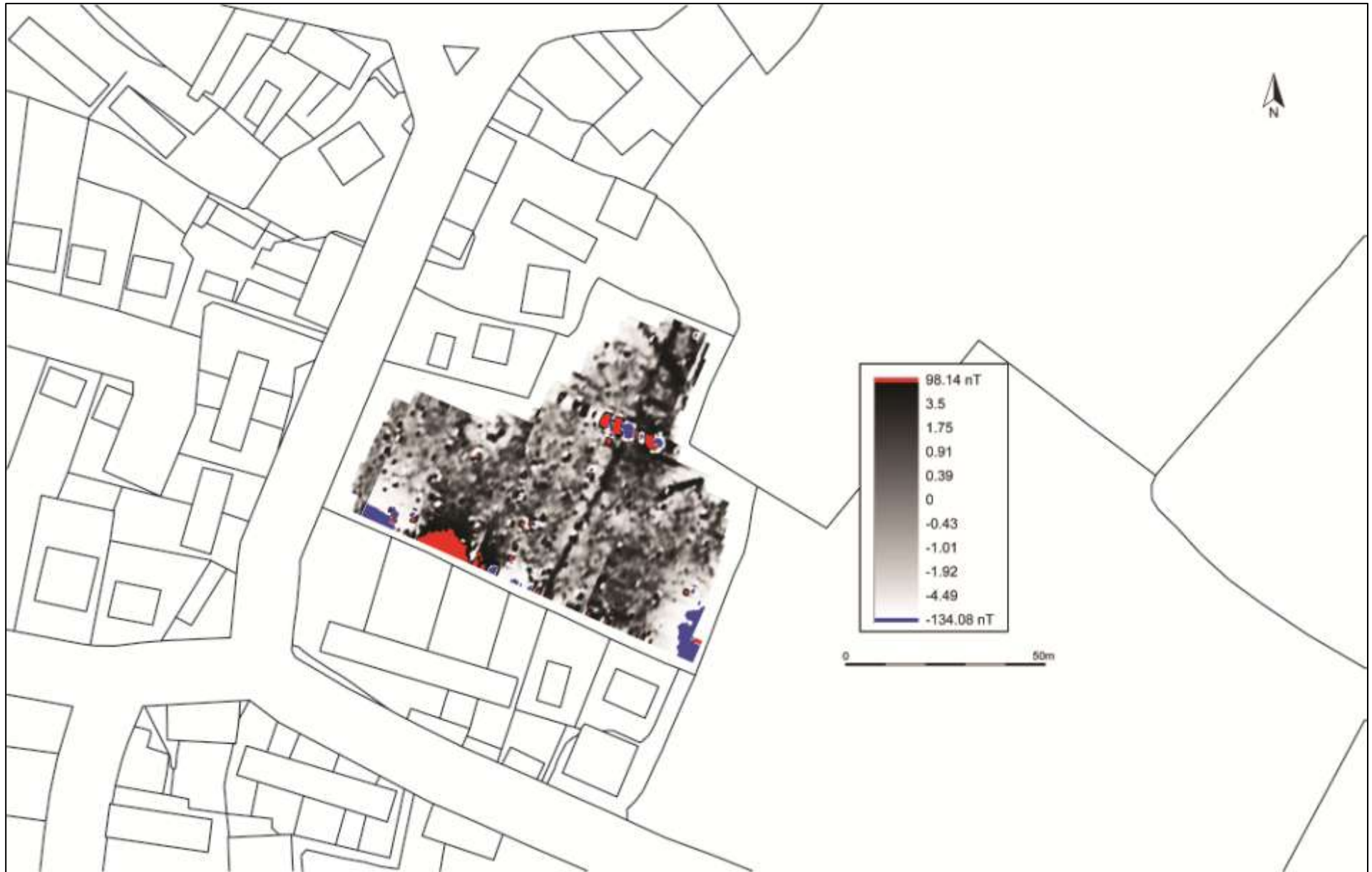
Red-Grey-Blue shade plot of gradiometer survey data; band weight equalised; gradiated shading.
