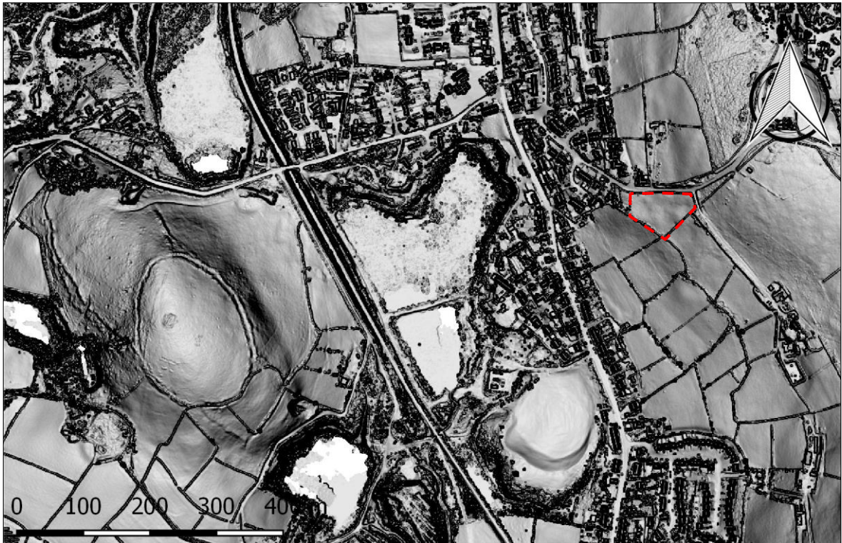
FIGURE 8: IMAGE DERIVED FROM 1M DSM LIDAR DATA, SHOWING THE SITE (INDICATED) (PROCESSED USING QGIS VER2.18.2, TERRAIN ANALYSIS/SLOPE, VERTICAL EXAGGERATION 3.0). DATA: © ENVIRONMENT AGENCY COPYRIGHT AND DATABASE RIGHTS 2017; CONTAINS OS DATA © CROWN COPYRIGHT AND DATABASE RIGHTS 2017. THE SITE IS INDICATED. NOTE THE HILLFORT AND ROUND TO THE LEFT OF THE IMAGE, AND THE LARGE ANNEX ON THE NORTH-WESTERN SIDE OF THE HILLFORT.
