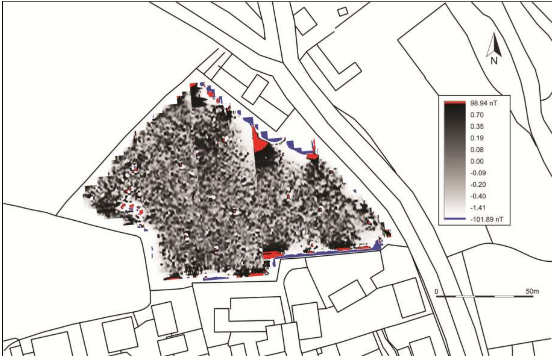
RED GREYSCALE BLUE SHADE PLOT OF GRADIOMETER SURVEY DATA; BAND WEIGHT EQUALISED; GRADIATED SHADING.
