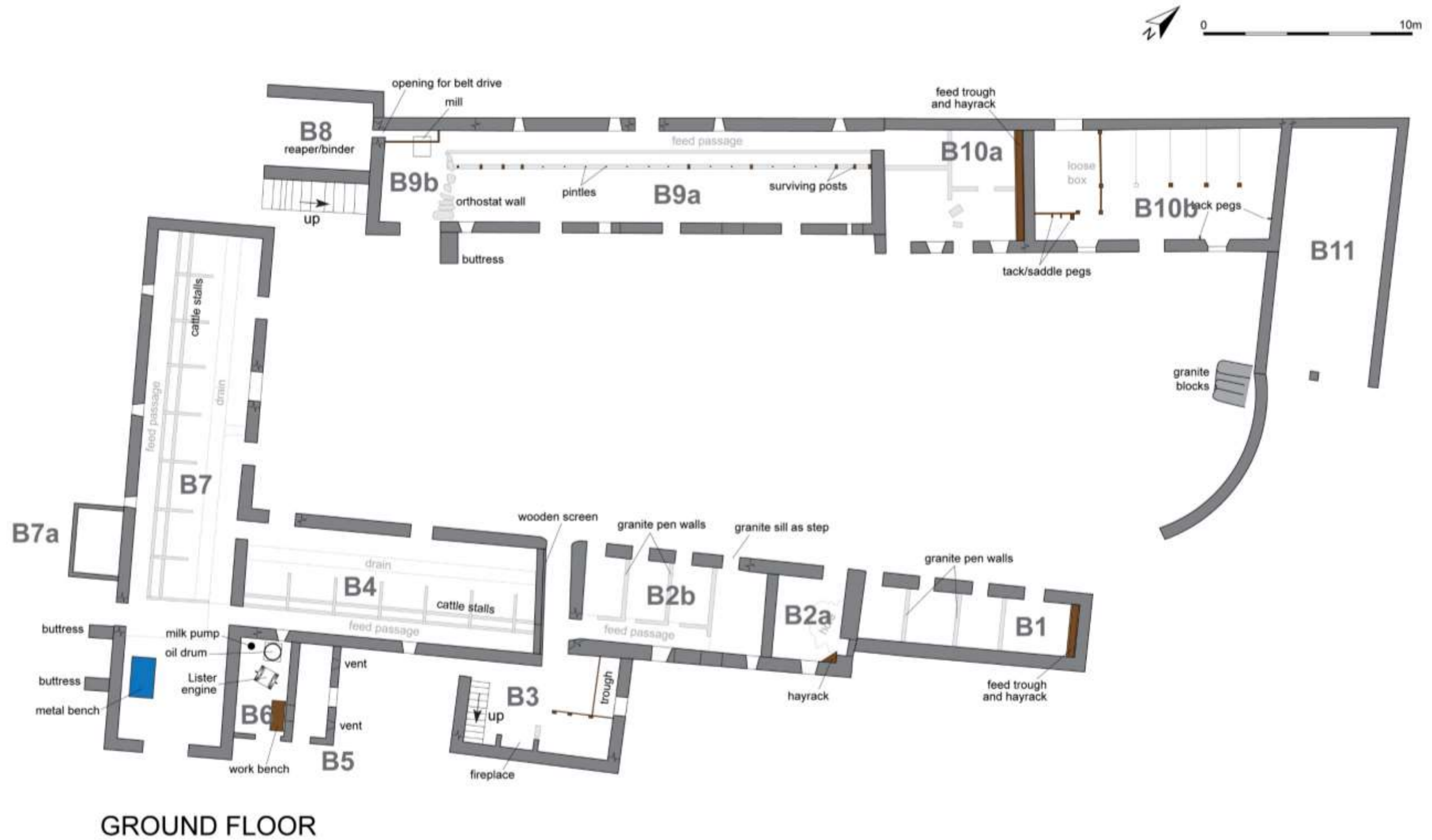
FIGURE 38: GROUND-FLOOR PLAN OF INTERNAL FEATURES (BASED ON SUPPLIED PLANS, SUPPLEMENTED BY A MEASURED SURVEY OF INTERNAL FEATURES).
