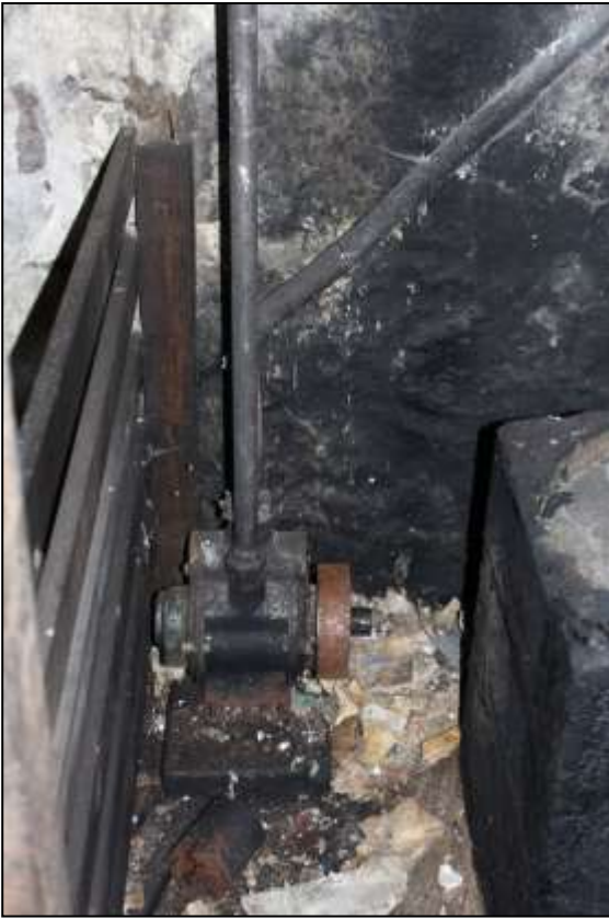
157. LEFT: B6 INTERIOR, DETAIL OF THE ALFA LAVAL MILK PUMP; VIEWED FROM THE SOUTH-EAST.
