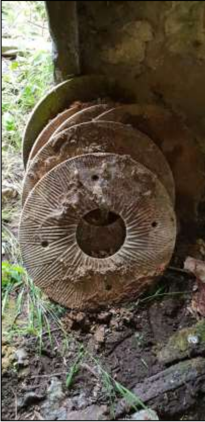
180. LEFT: B9b GF INTERIOR, DETAIL OF EX SITU GRINDING PLATES FROM A BURR MILL; VIEWED FROM THE NORTH-WEST.
