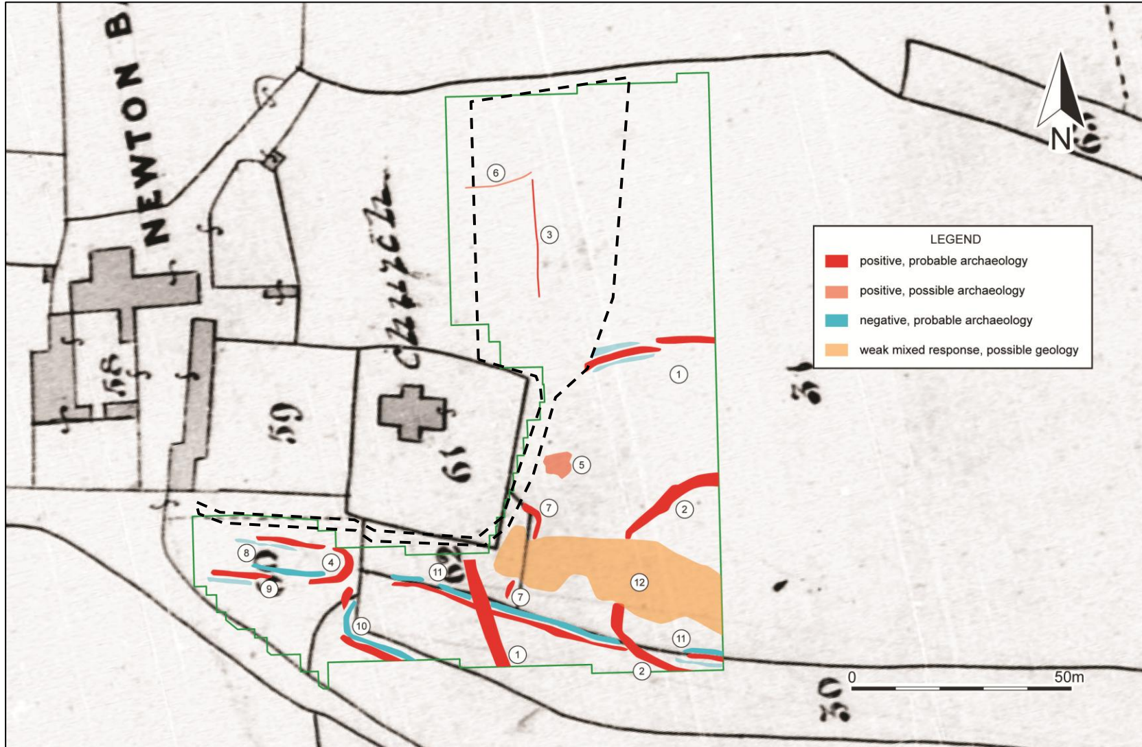
FIGURE 12: INTERPRETATION OF GRADIOMETER SURVEY DATA. THE SITE IS OUTLINED WITH A DASHED BLACK LINE.
