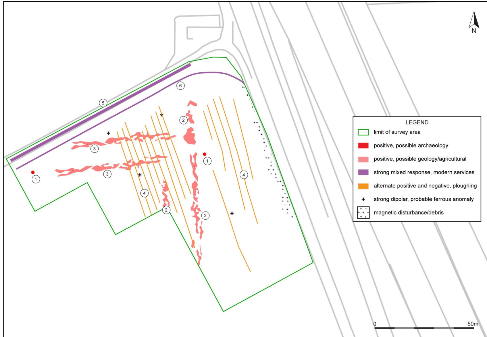
FIGURE 13: INTERPRETATION OF GRADIOMETER SURVEY DATA.
