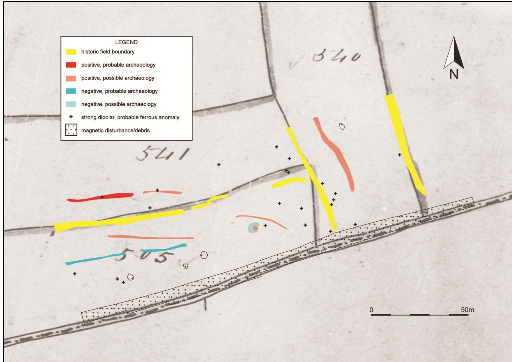
FIGURE 9: INTERPRETATION OF GRADIOMETER SURVEY DATA OVERLYING 1841 SHOBROOKE TITHE MAPPING.
