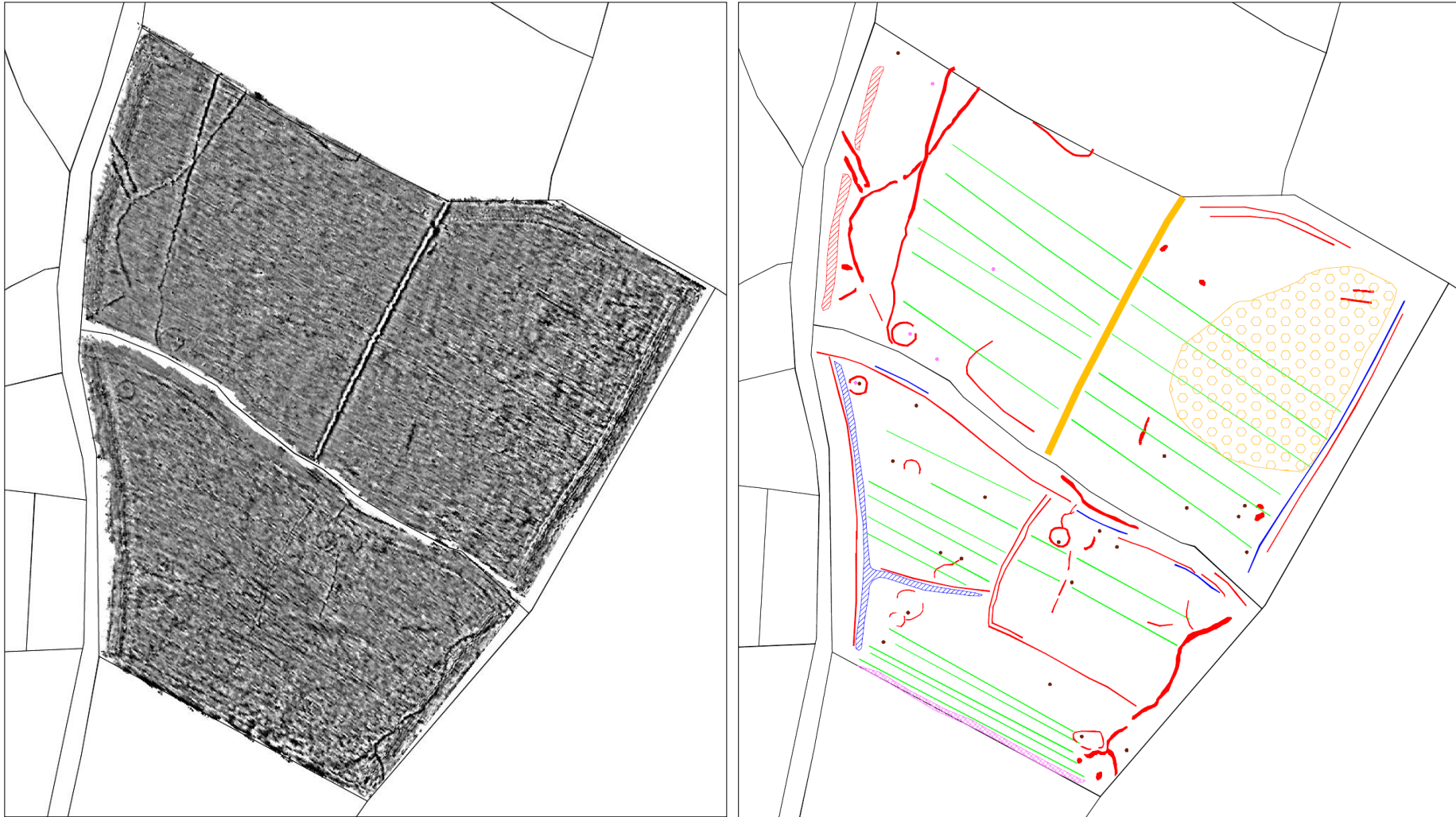
LEFT: FIGURE 6: PLOT OF THE CARINES FARM SOLAR FARM PROCESSED GRADIOMETER DATA (STRATASCAN 2011, FIG.11).
