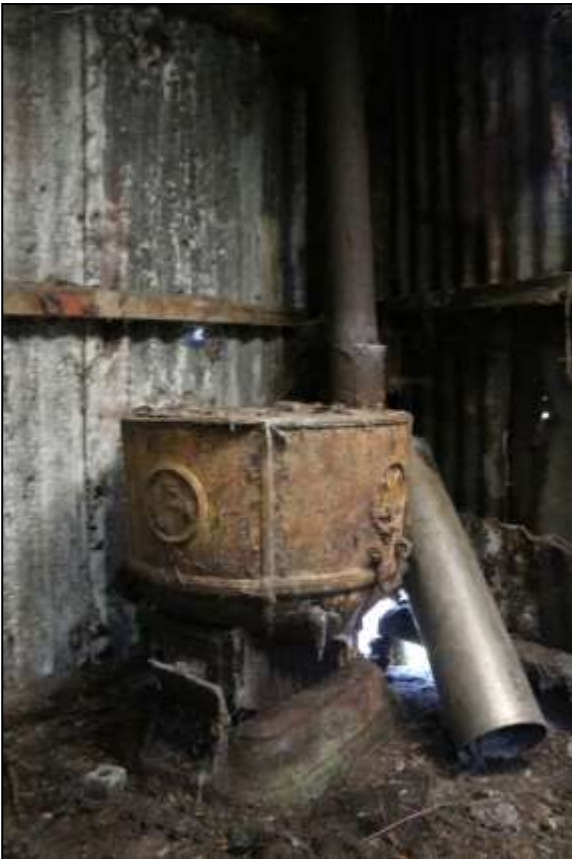
44. AS ABOVE, DETAIL OF THE SWILL BOILER; VIEWED FROM THE SOUTH.
