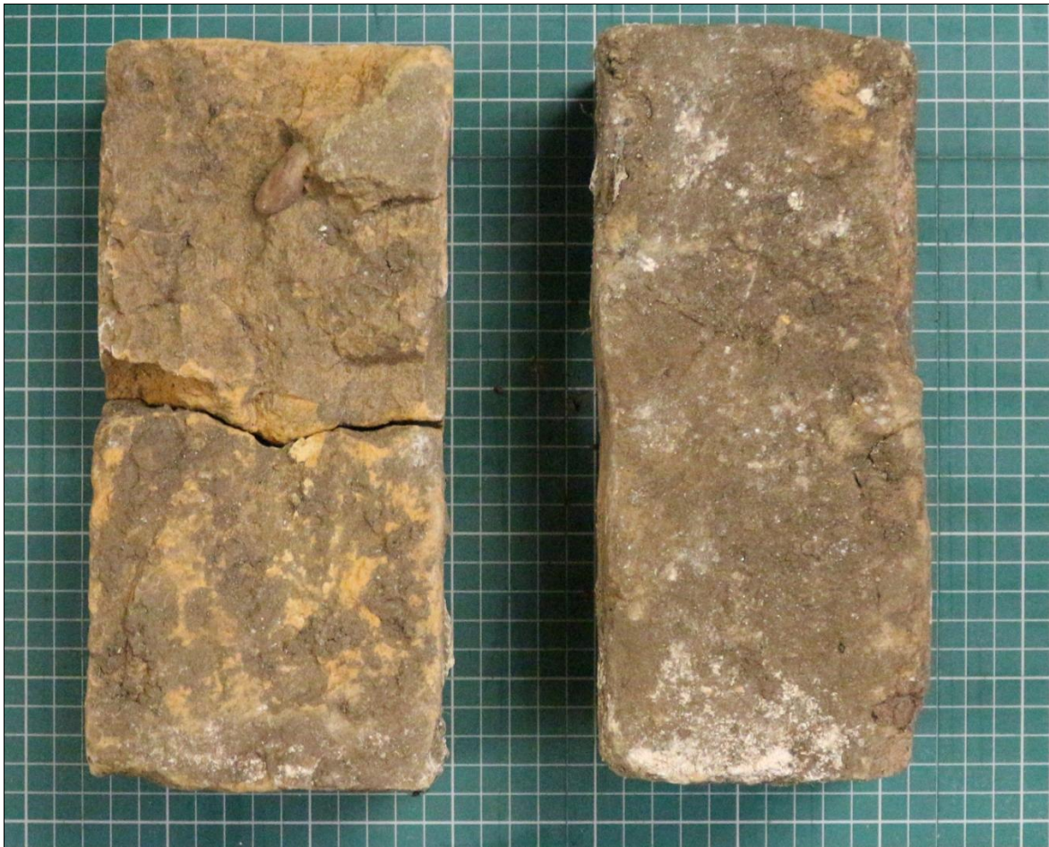
FIGURE 8: EXAMPLES OF THE TWO KINDS OF BRICK ENCOUNTERED (10MM SCALE IN BACKGROUND).
