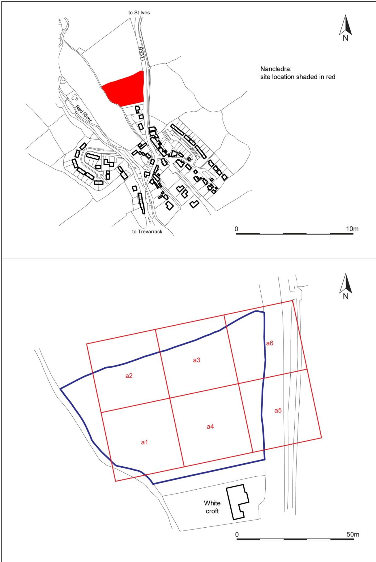
FIGURE 3: (ABOVE) SITE LOCATION IN NANCLEDRA; (BELOW) GEOPHYSICAL SURVEY GRID LOCATION AND NUMBERING.
