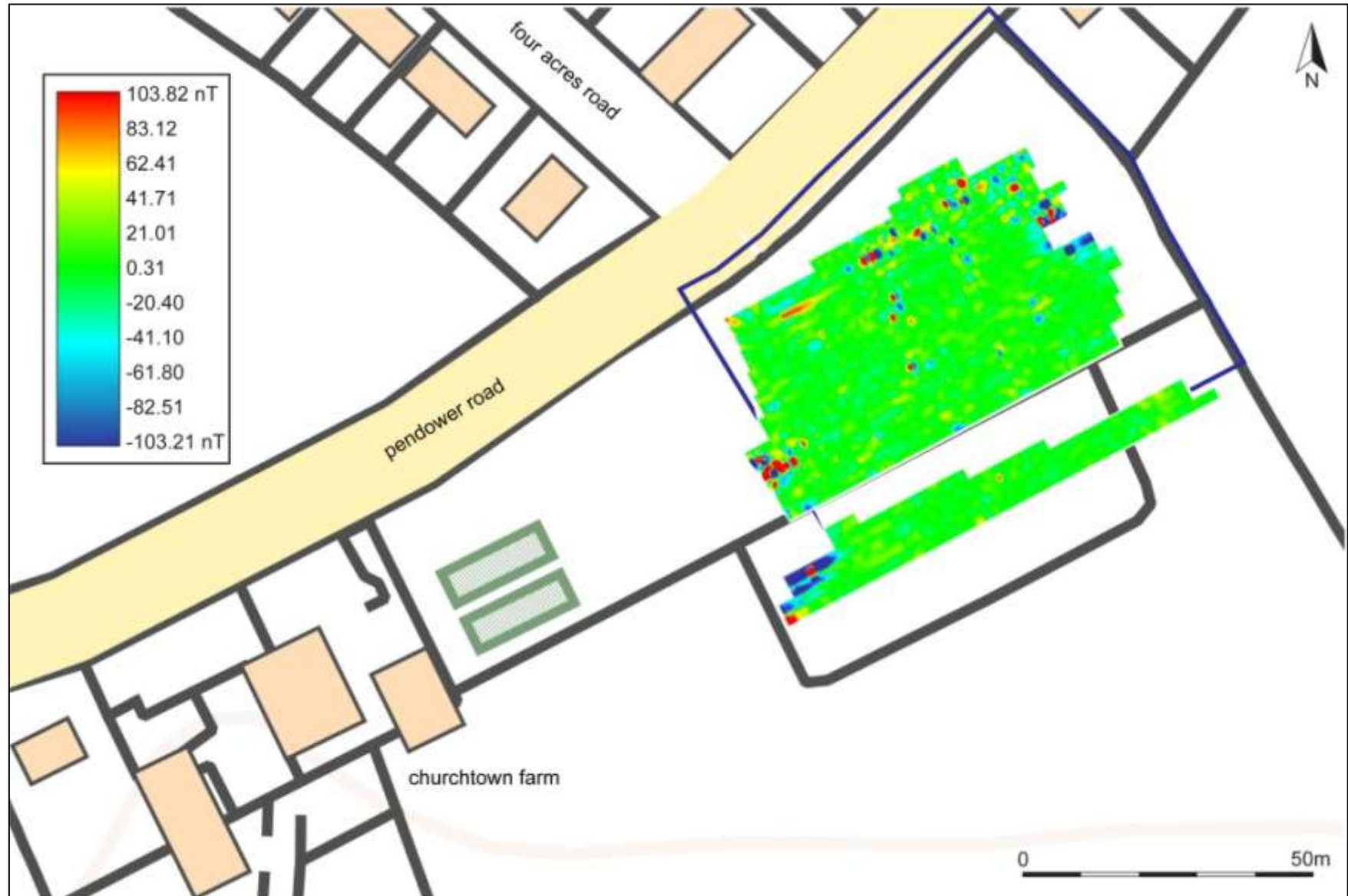
FIGURE 6: RED-BLUE-GREEN2 SHADE PLOT OF GRADIOMETER SURVEY DATA; GRADIATED SHADING.
