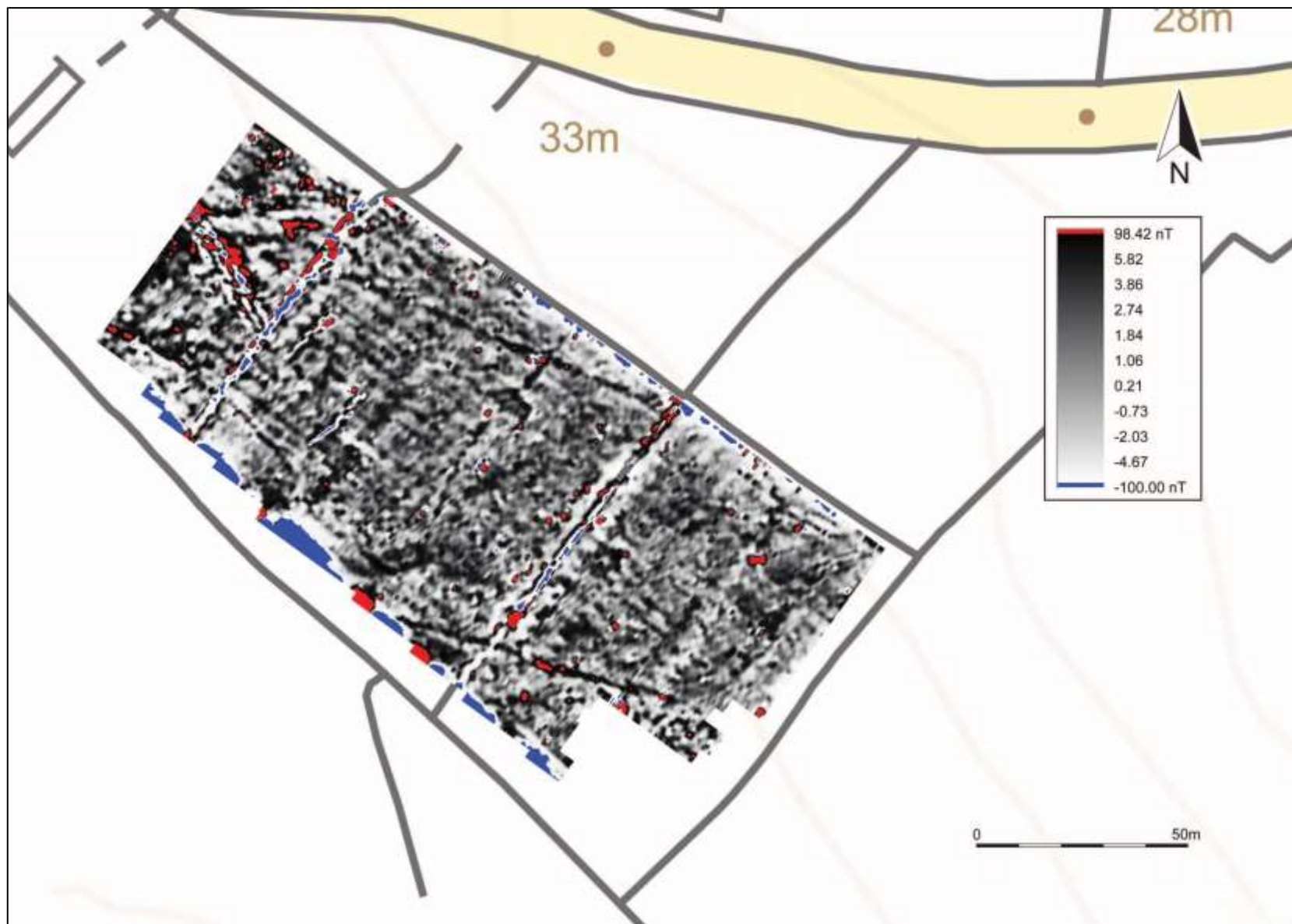
FIGURE 9: RED GREYSCALE BLUE SHADE PLOT OF GRADIOMETER SURVEY DATA; BAND WEIGHT EQUALISED; GRADIATED SHADING.
