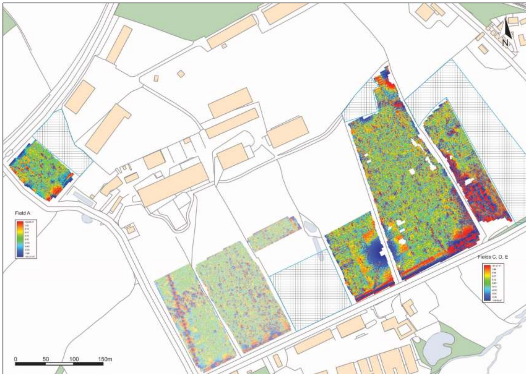
RED-BLUE-GREEN(2) SHADE PLOT OF GRADIOMETER SURVEY DATA; BAND WEIGHT EQUALISED; GRADIATED SHADING.
