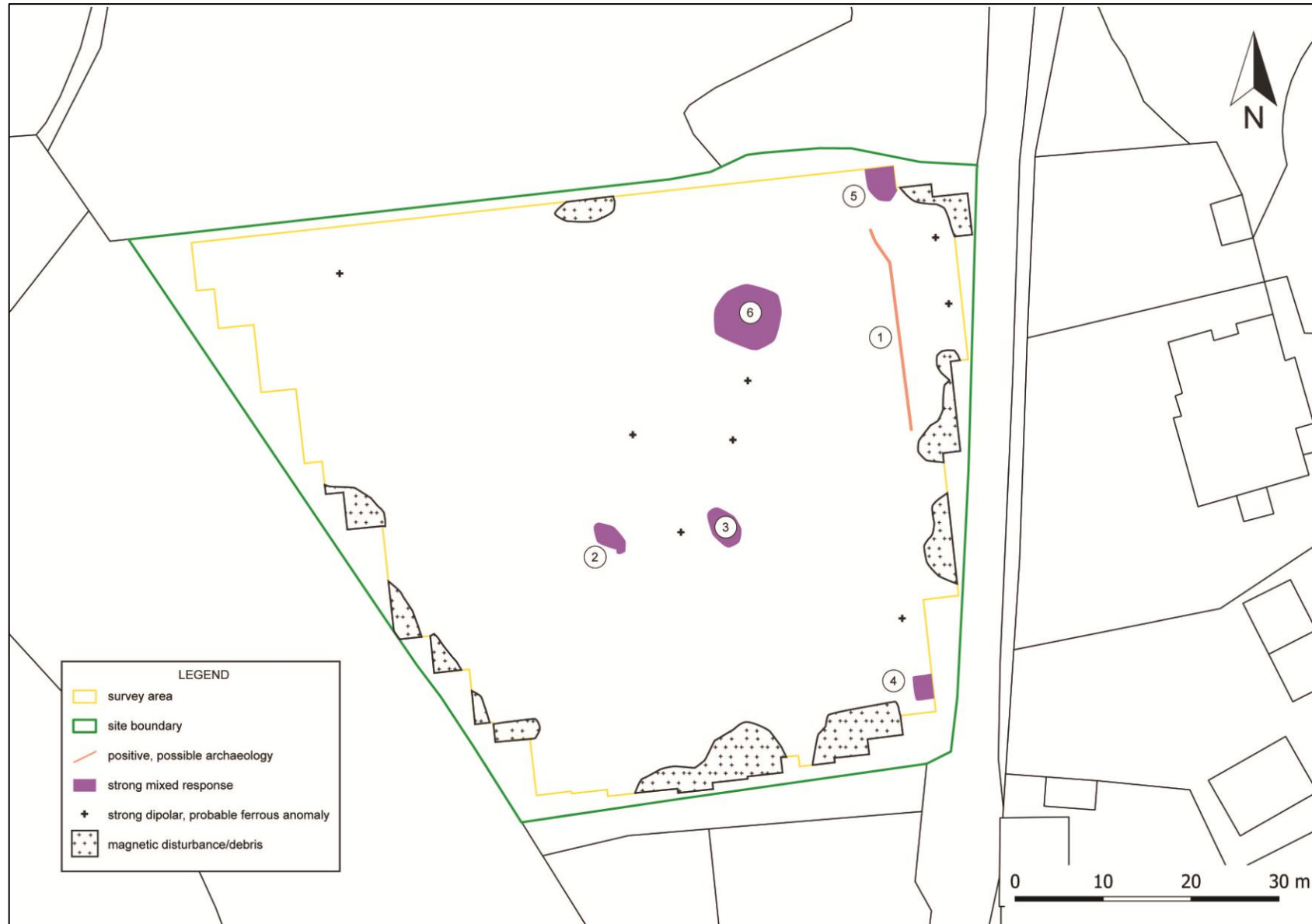
FIGURE 6: INTERPRETATION OF GRADIOMETER SURVEY DATA.
