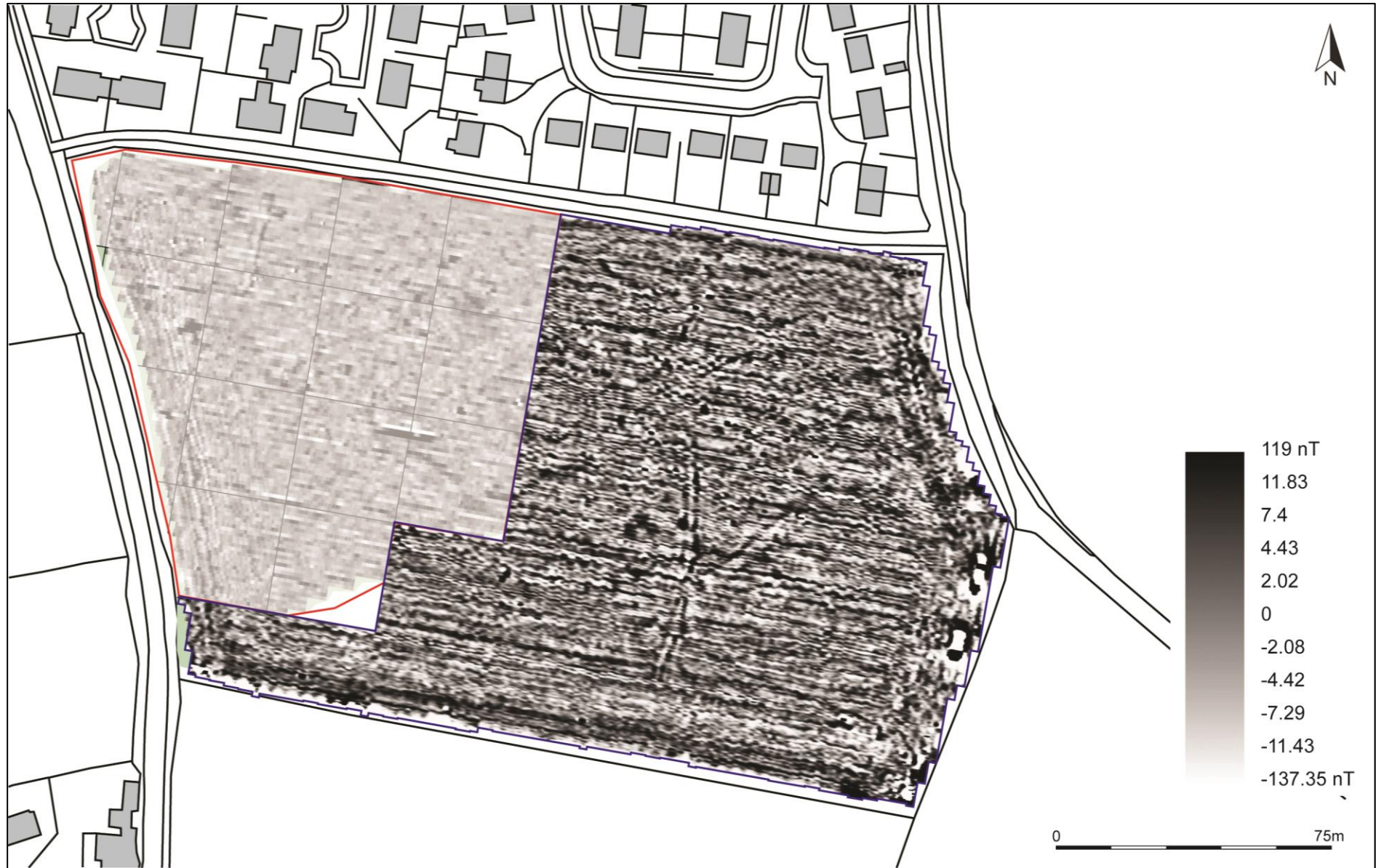
SHADE PLOT OF GRADIOMETER SURVEY DATA; GRADIATED SHADING, BAND WEIGHT EQUALISED (2017 SURVEY OUTLINED IN RED; 2019 SURVEY OUTLINED IN BLUE).
