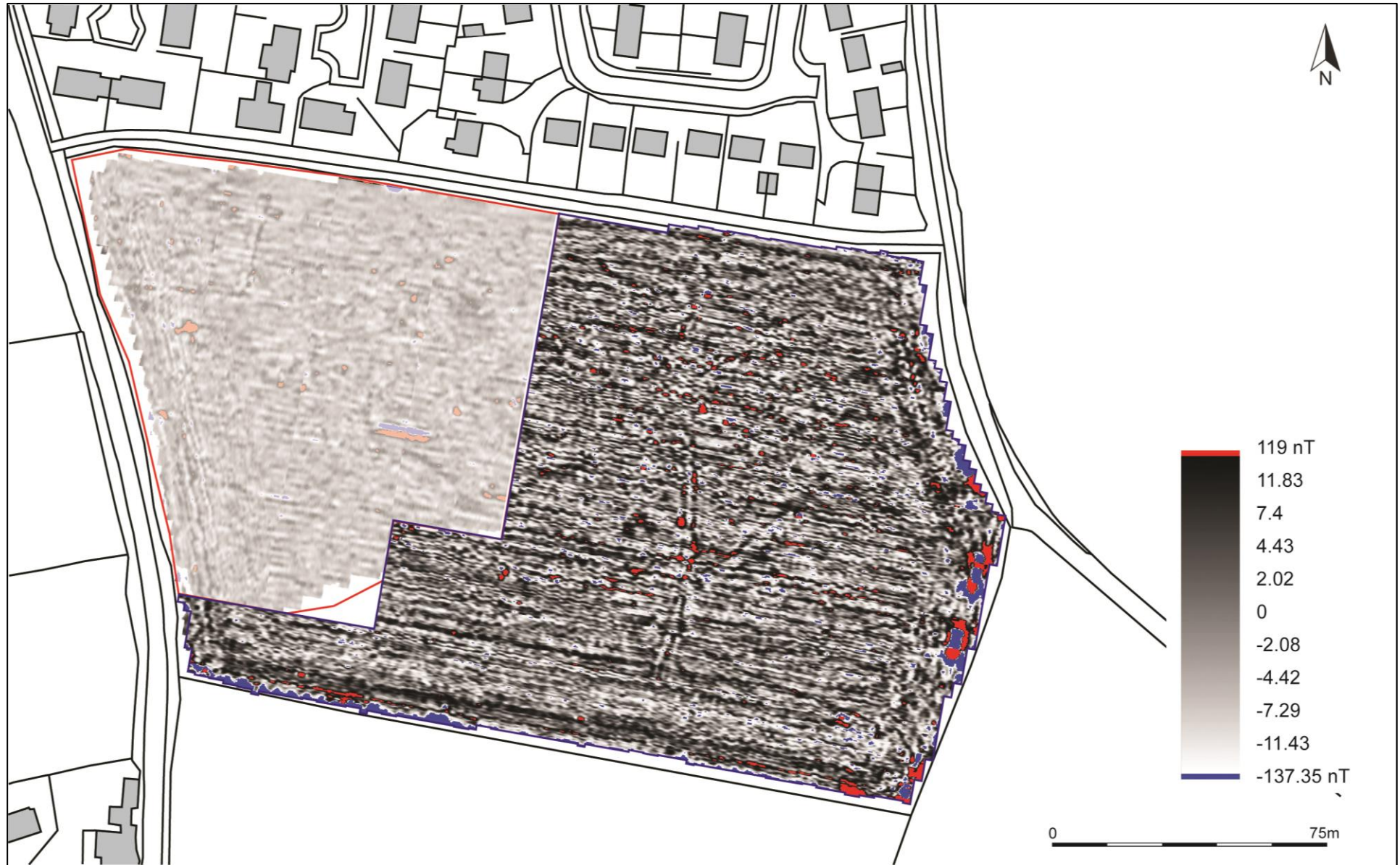
RED GREYSCALE BLUE SHADE PLOT OF GRADIOMETER SURVEY DATA; GRADIATED SHADING, BAND WEIGHT EQUALISED (2017 SURVEY OUTLINED IN RED; 2019 SURVEY OUTLINED IN BLUE).
