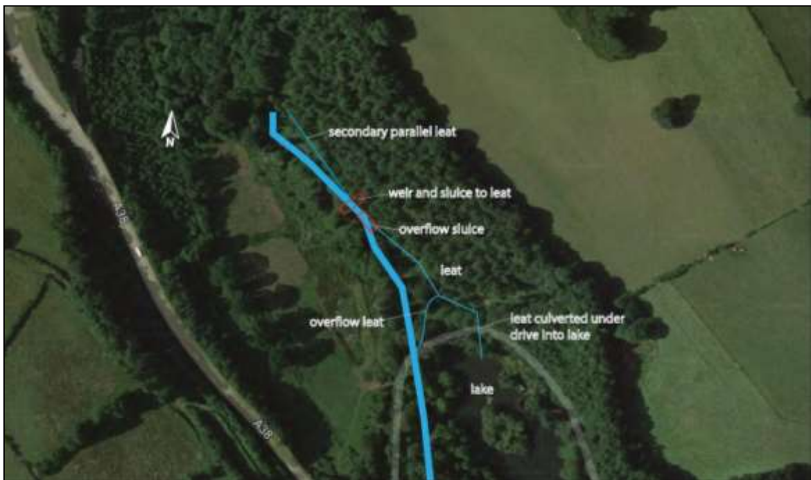
FIGURE 2: ANNOTATED AERIAL IMAGE INDICATING THE WEIR AND LEAT SYSTEMS.
