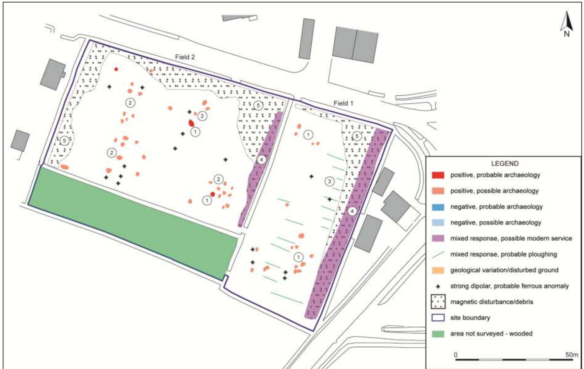
FIGURE 10: INTERPRETATION OF GRADIOMETER SURVEY DATA (SITE BOUNDARY OUTLINED IN BLUE).
