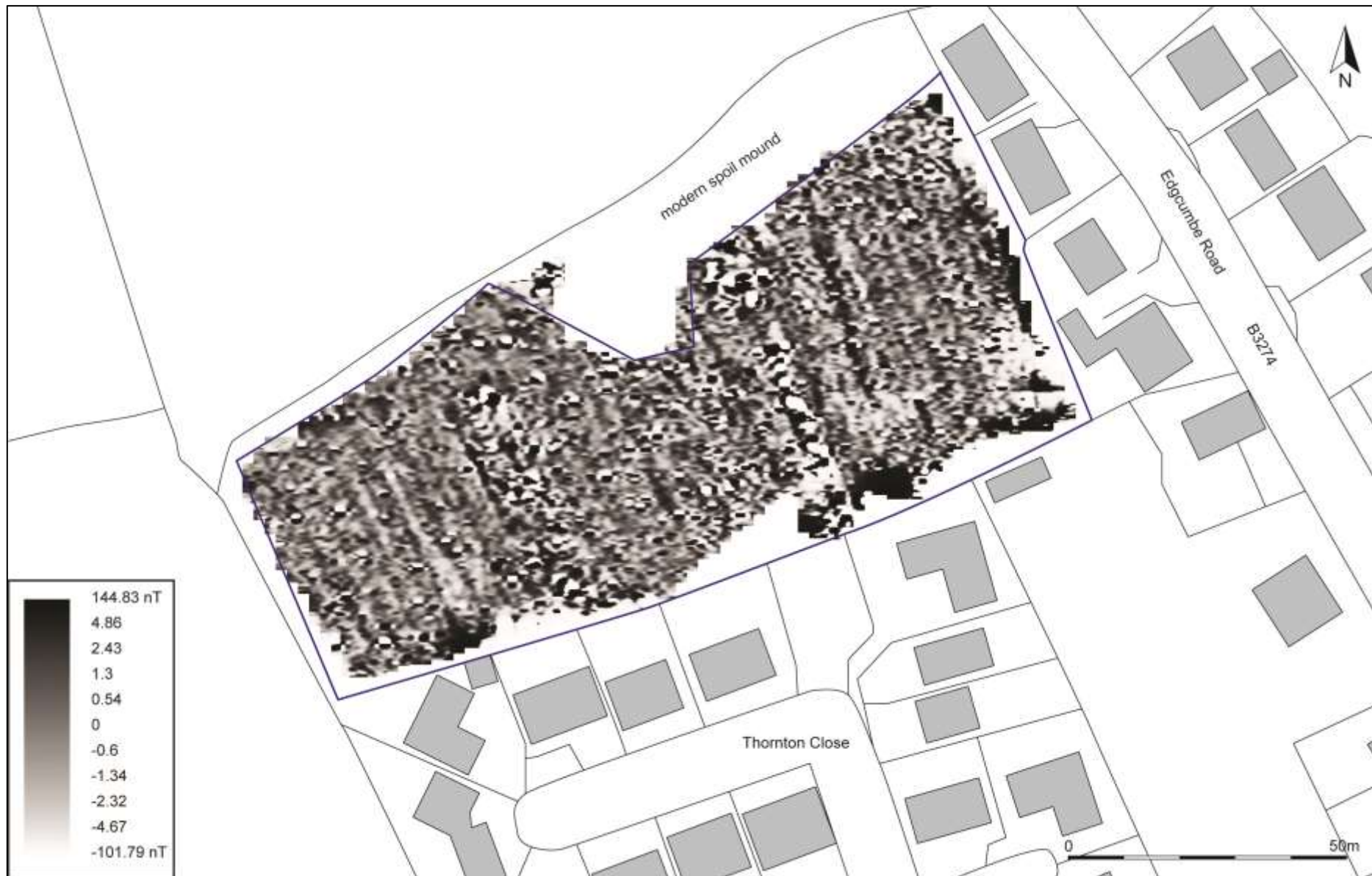
FIGURE 8: SHADE PLOT OF GRADIOMETER SURVEY DATA; BAND WEIGHT EQUALISED, GRADIATED SHADING (SITE BOUNDARY OUTLINED IN BLUE).
