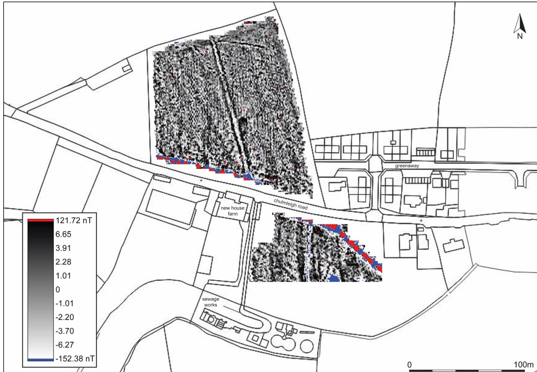
FIGURE 10: RED-GREY-BLUE SHADE PLOT OF GRADIOMETER SURVEY DATA; BAND WEIGHT EQUALISED; GRADIATED SHADING.
