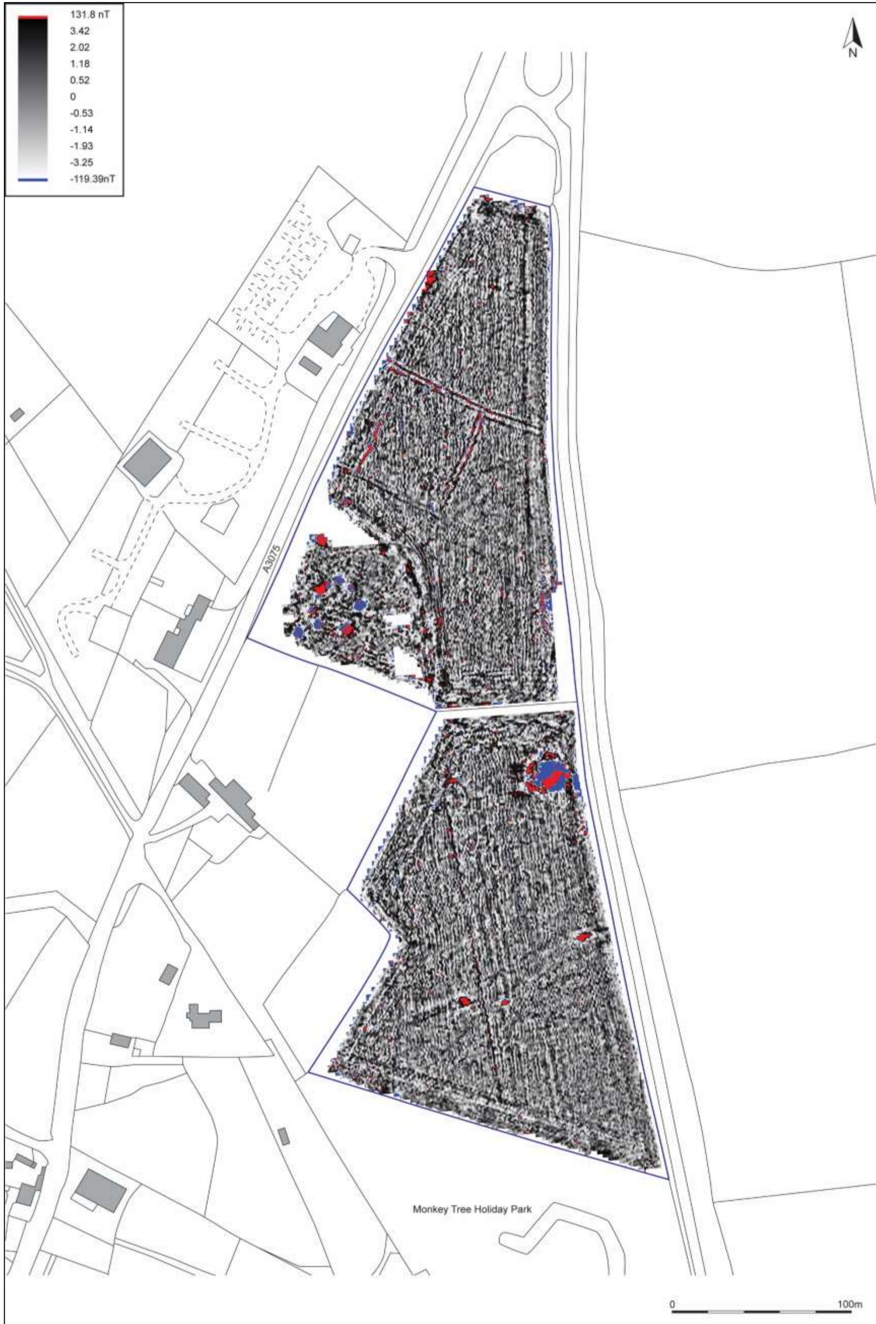
RED GREYSCALE BLUE SHADE PLOT OF GRADIOMETER SURVEY DATA; BAND WEIGHT EQUALISED, GRADIATED SHADING.
