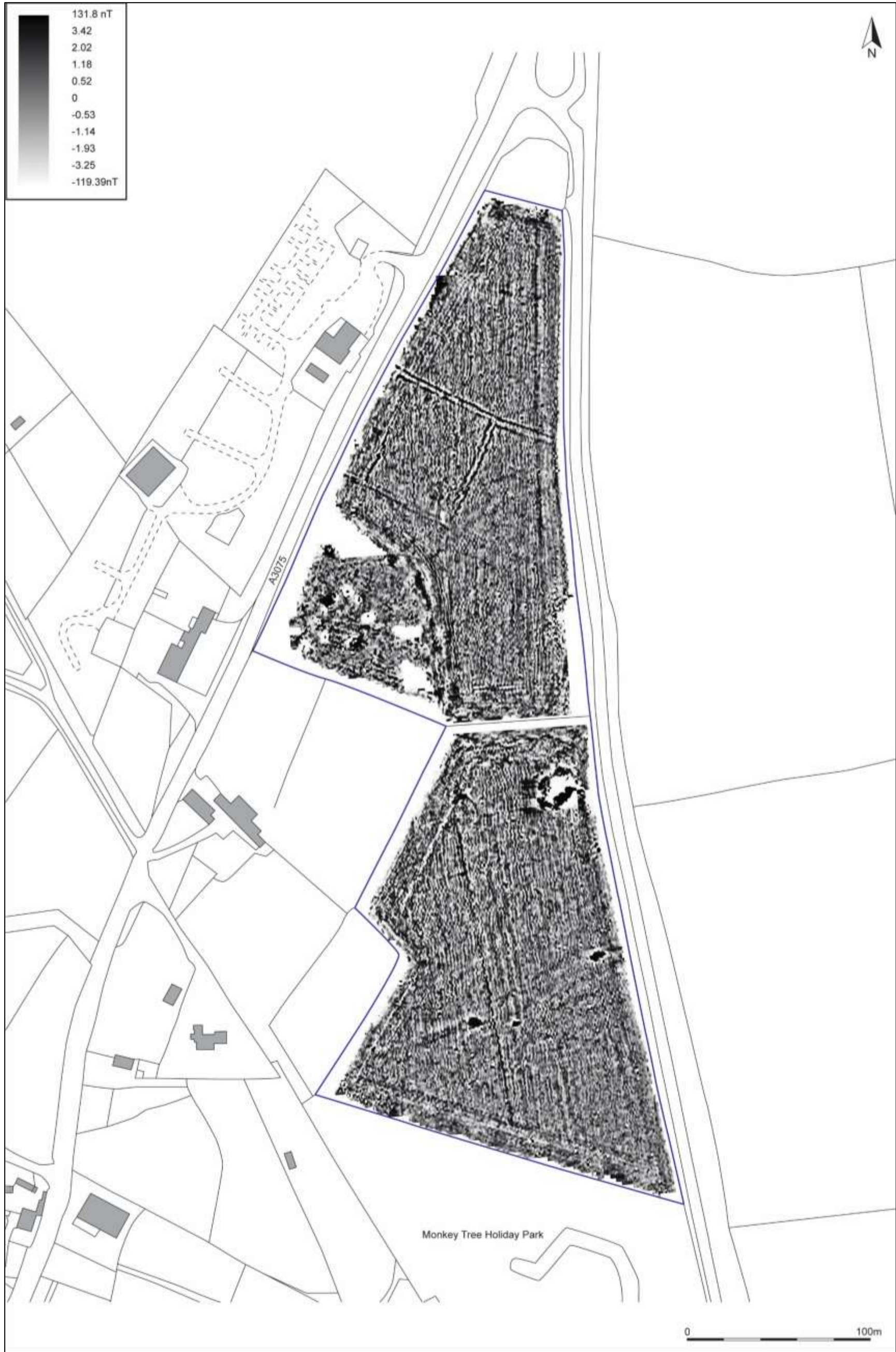
FIGURE 12: SHADE PLOT OF GRADIOMETER SURVEY DATA; BANDWEIGHT EQUALISED, GRADIATED SHADING.
