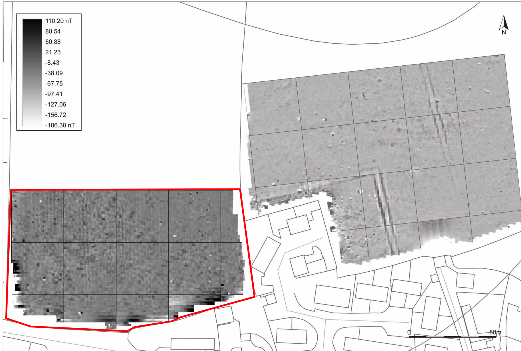
FIGURE 2: SHADE PLOT OF GRADIOMETER SURVEY DATA; MINIMAL PROCESSING (BOUNDED IN RED). RESULTS OF THE ADJACENT 2018 SURVEY ARE ALSO SHOWN.
