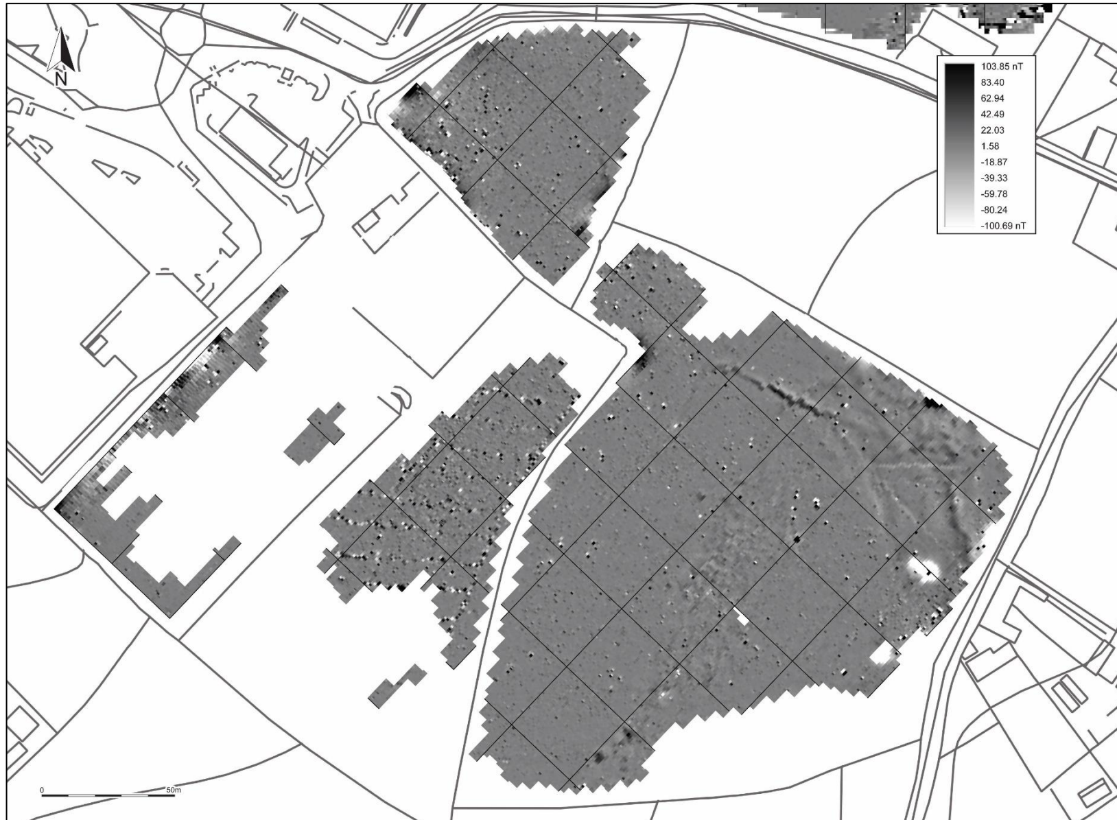
FIGURE 12: SHADE PLOT OF GRADIOMETER SURVEY DATA; GREYSCALE; FIELDS G-J.
