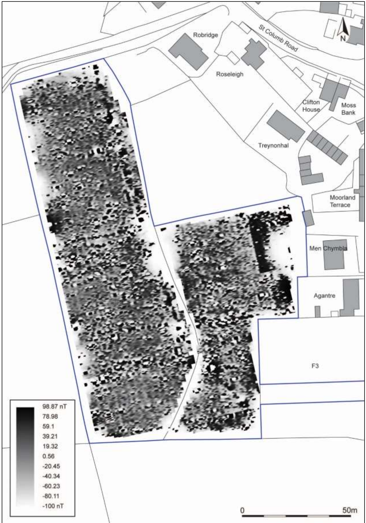
FIGURE 9: SHADE PLOT OF GRADIOMETER SURVEY DATA; MINIMAL PROCESSING (SITE BOUNDARY OUTLINED IN BLUE).
