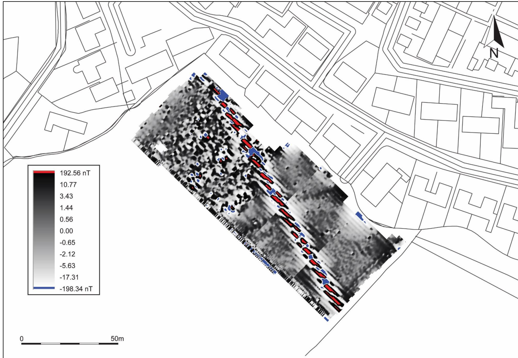
FIGURE 15: RED GREYSCALE BLUE SHADE PLOT OF GRADIOMETER SURVEY DATA; BAND WEIGHT EQUALISED; GRADIATED SHADING.
