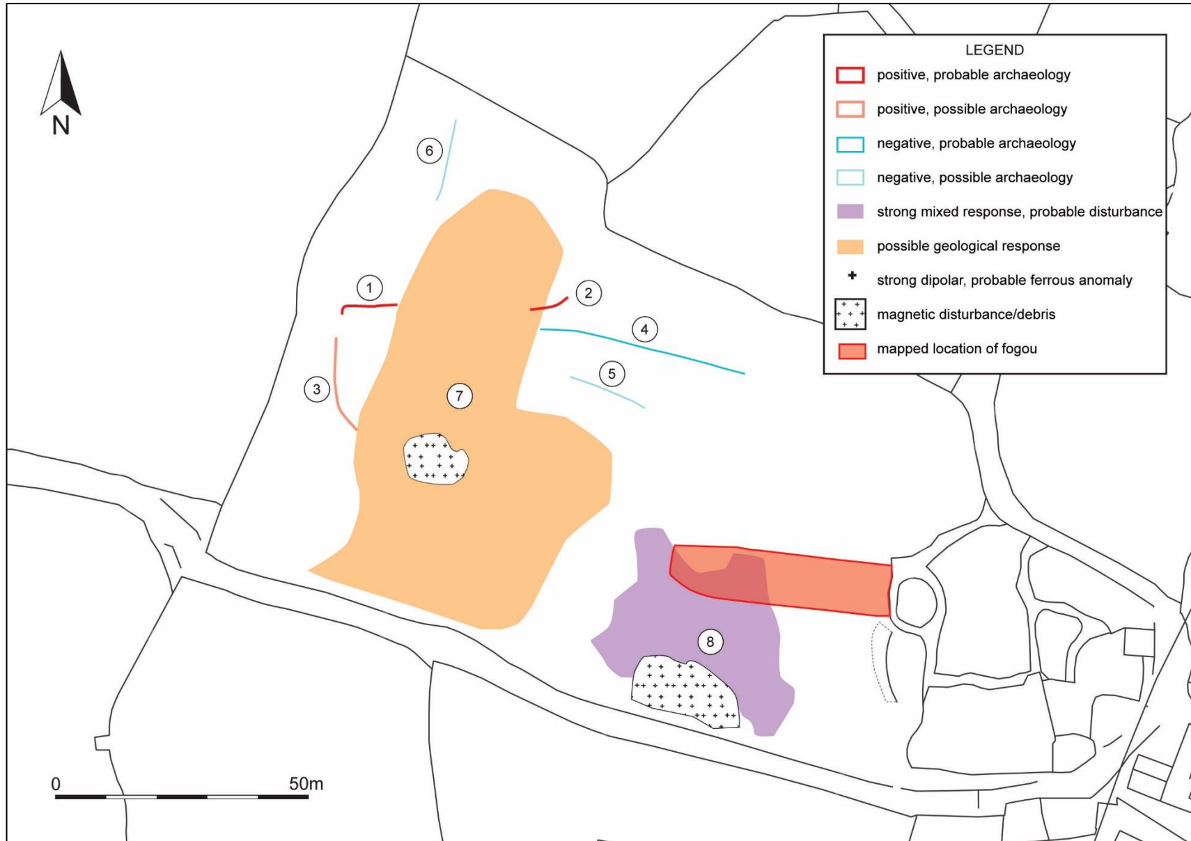
FIGURE 9: INTERPRETATION OF THE GRADIOMETER SURVEY DATA.
