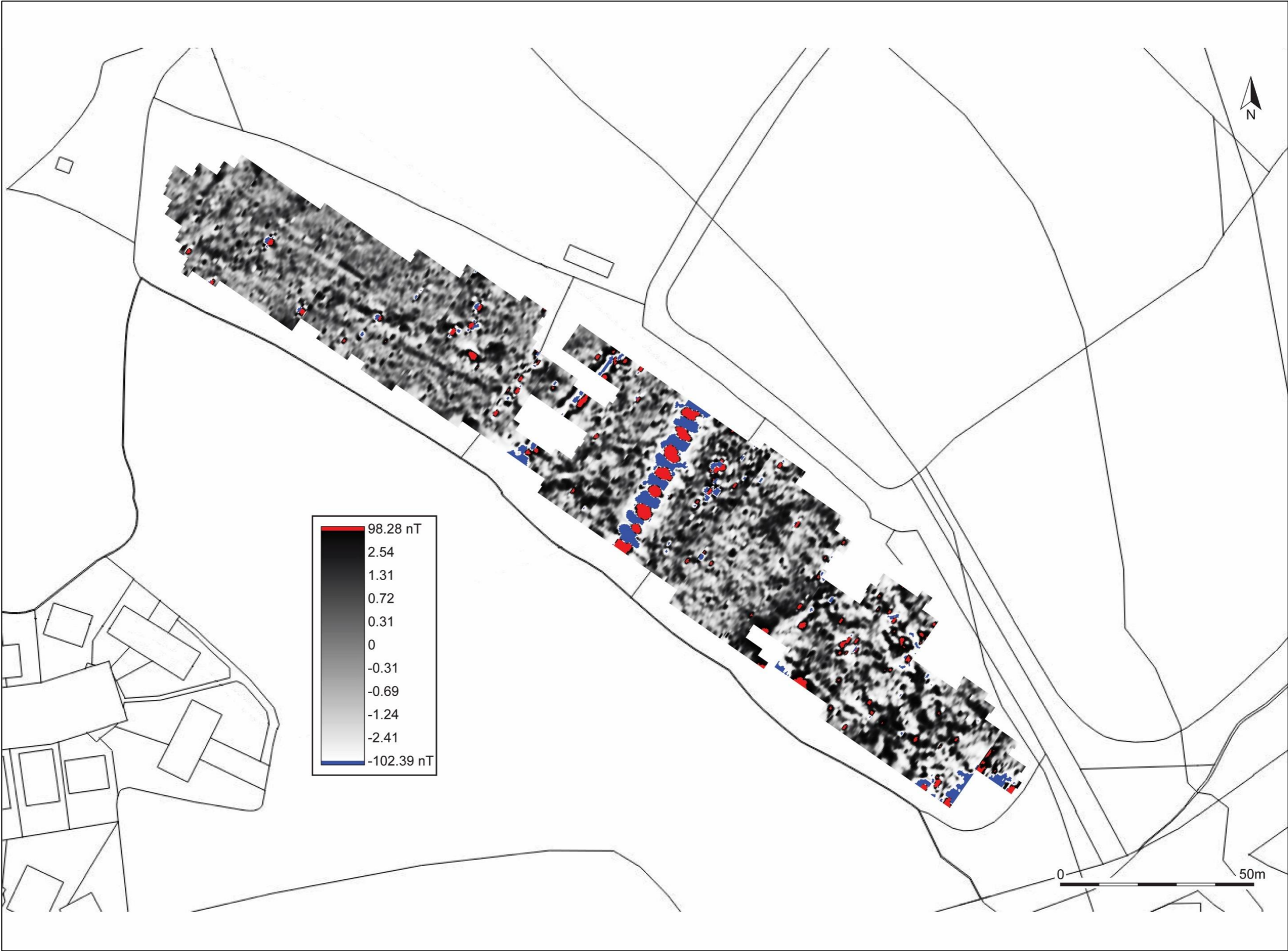
FIGURE 5: RED-GREY-BLUE SHADE PLOT OF GRADIOMETER SURVEY DATA; BAND WEIGHT EQUALISED; GRADIATED SHADING.
