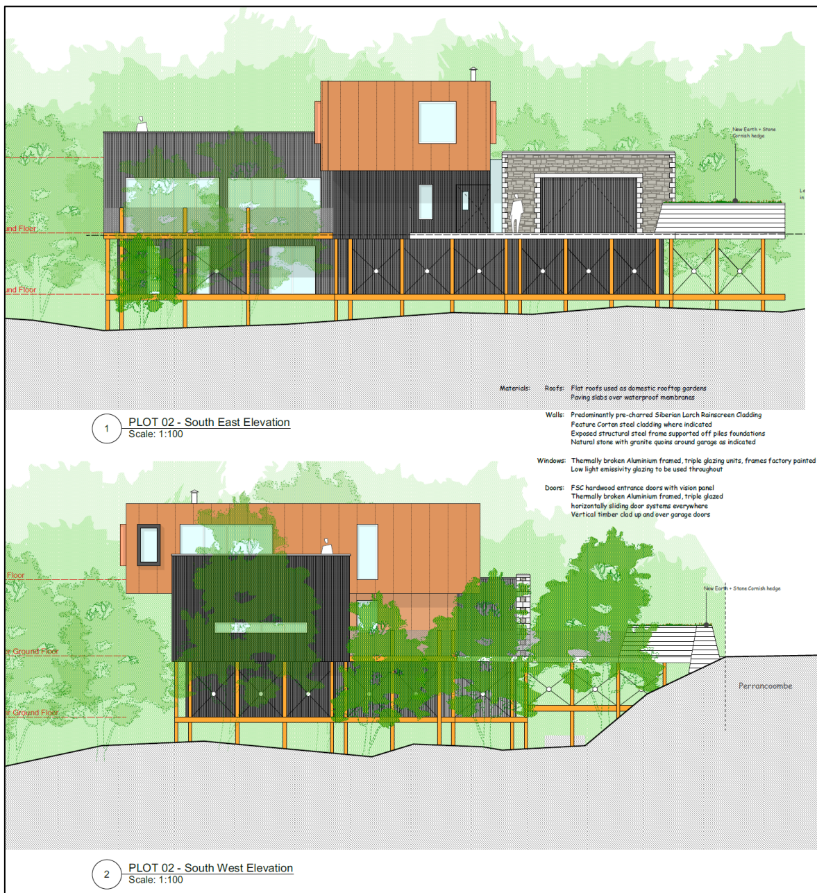
FIGURE 13: ELEVATIONS OF THE PLOT02 HOUSE, SHOWING THE PILED STRUCTURE (SUPPLIED BY AGENT).
