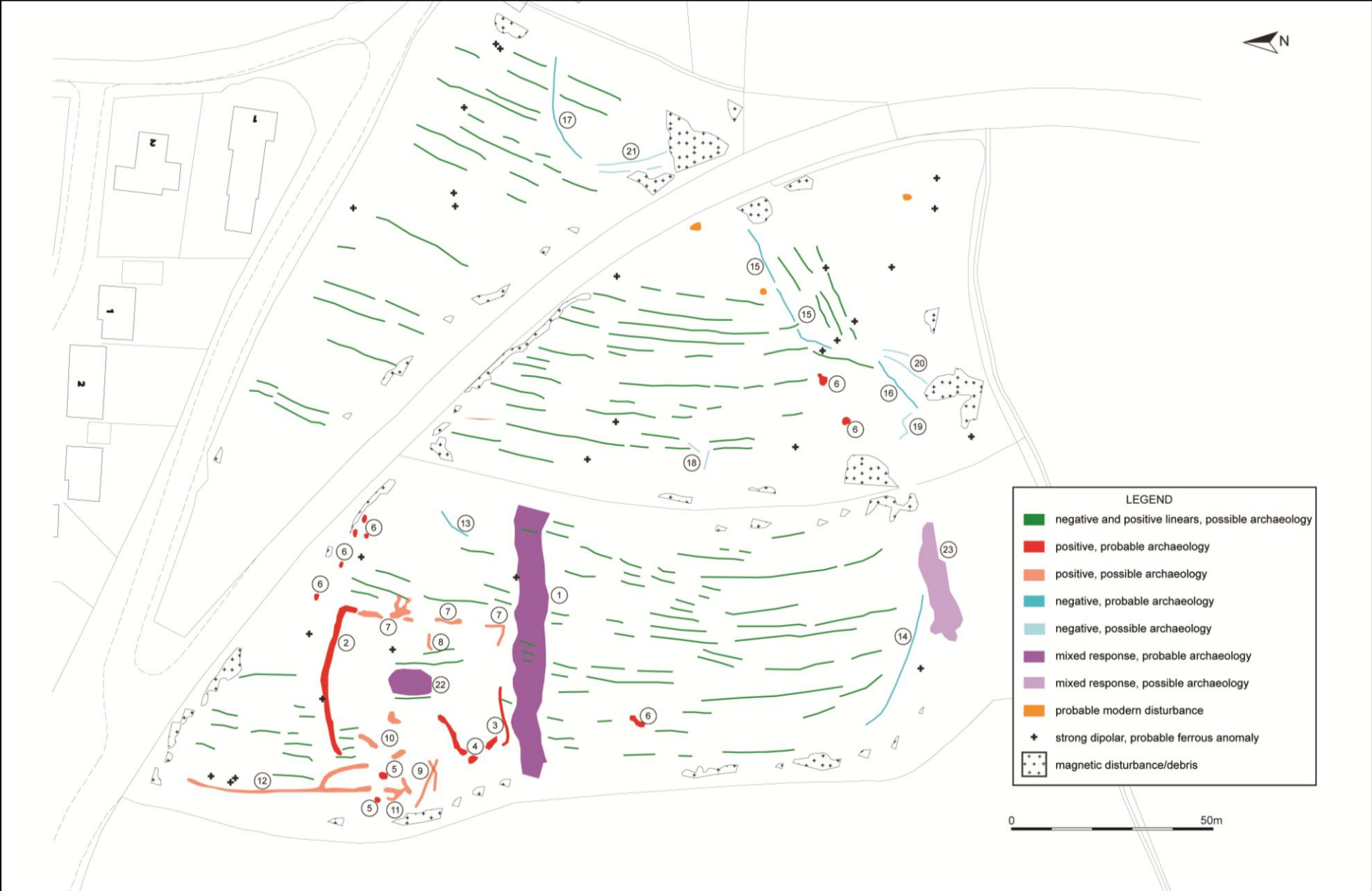
FIGURE 16: INTERPRETATION OF GRADIOMETER SURVEY DATA.
