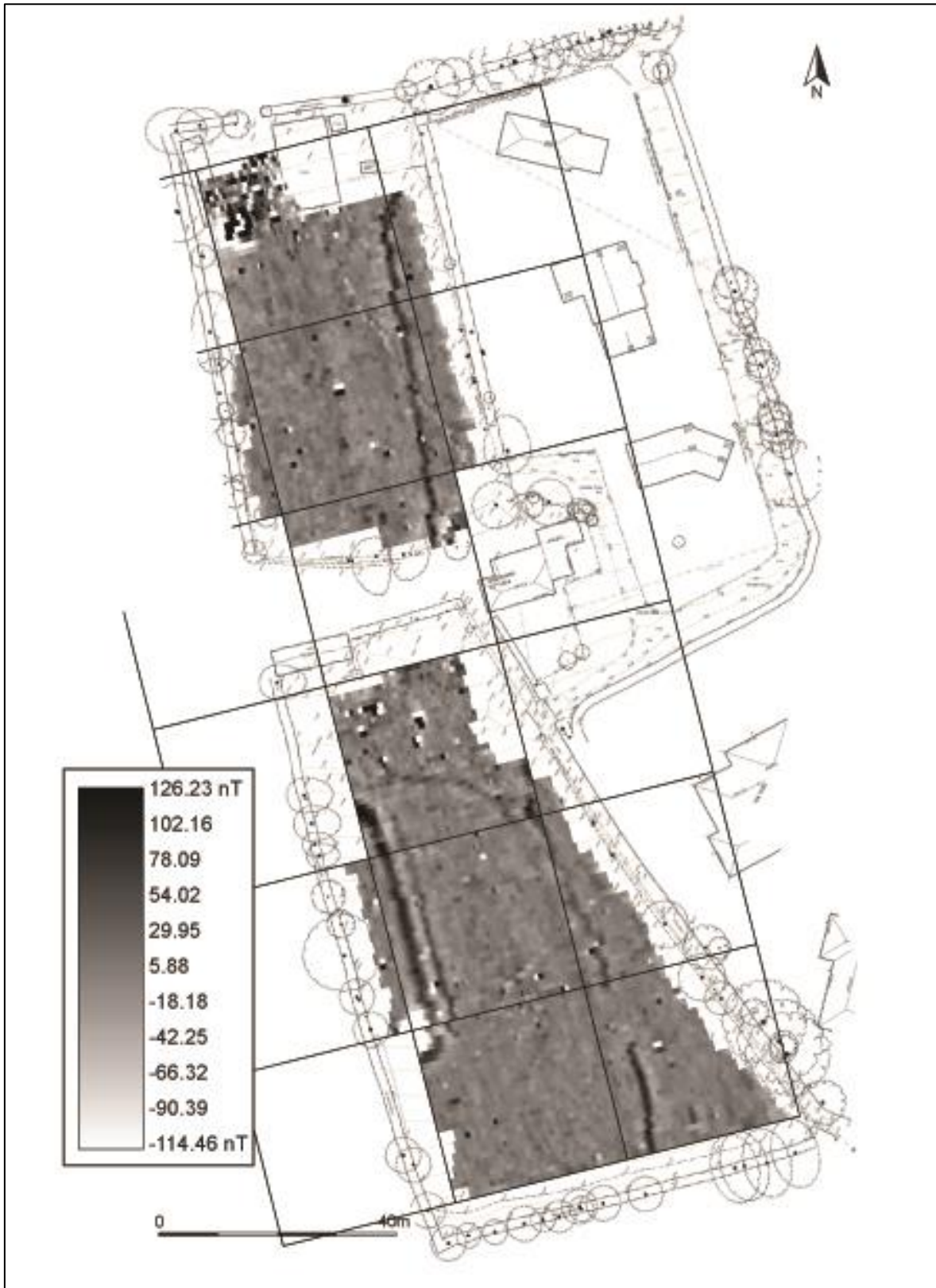
FIGURE 2: SHADE PLOT OF GRADIOMETER SURVEY DATA; MINIMAL PROCESSING.
