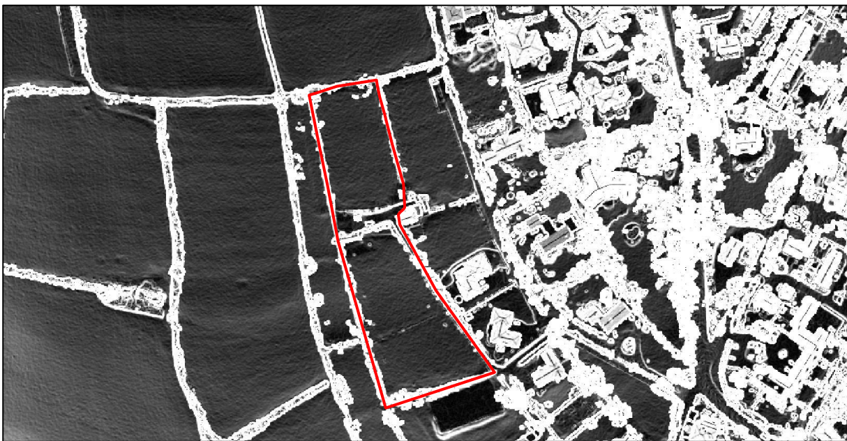
FIGURE 13: IMAGE DERIVED FROM LIDAR DATA; THE SITE IS OUTLINED IN RED (PROCESSED USING QGIS VER2.18.4, TERRAIN ANALYSIS/SLOPE, VERTICAL EXAGGERATION 3.0). DATA: CONTAINS FREELY AVAILABLE DATA SUPPLIED BY NATURAL ENVIRONMENT RESEARCH COUNCIL (CENTRE FOR ECOLOGY & HYDROLOGY; BRITISH ANTARCTIC SURVEY; BRITISH GEOLOGICAL SURVEY); ©NERC.
