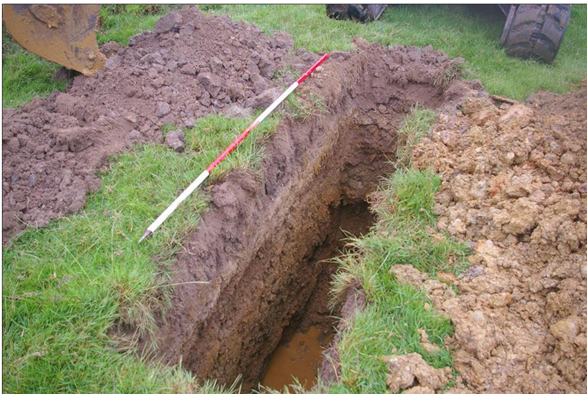
FIGURE 4: TRIAL-PIT 02, NORTH-EAST FACING SECTION DEMONSTRATING THE 'DRY' UPSLOPE DEPOSITS OVER RIVER GRAVELS OF THE NORTHERN EDGE OF THE SITE; VIEWED FROM THE EAST (2M SCALE).
