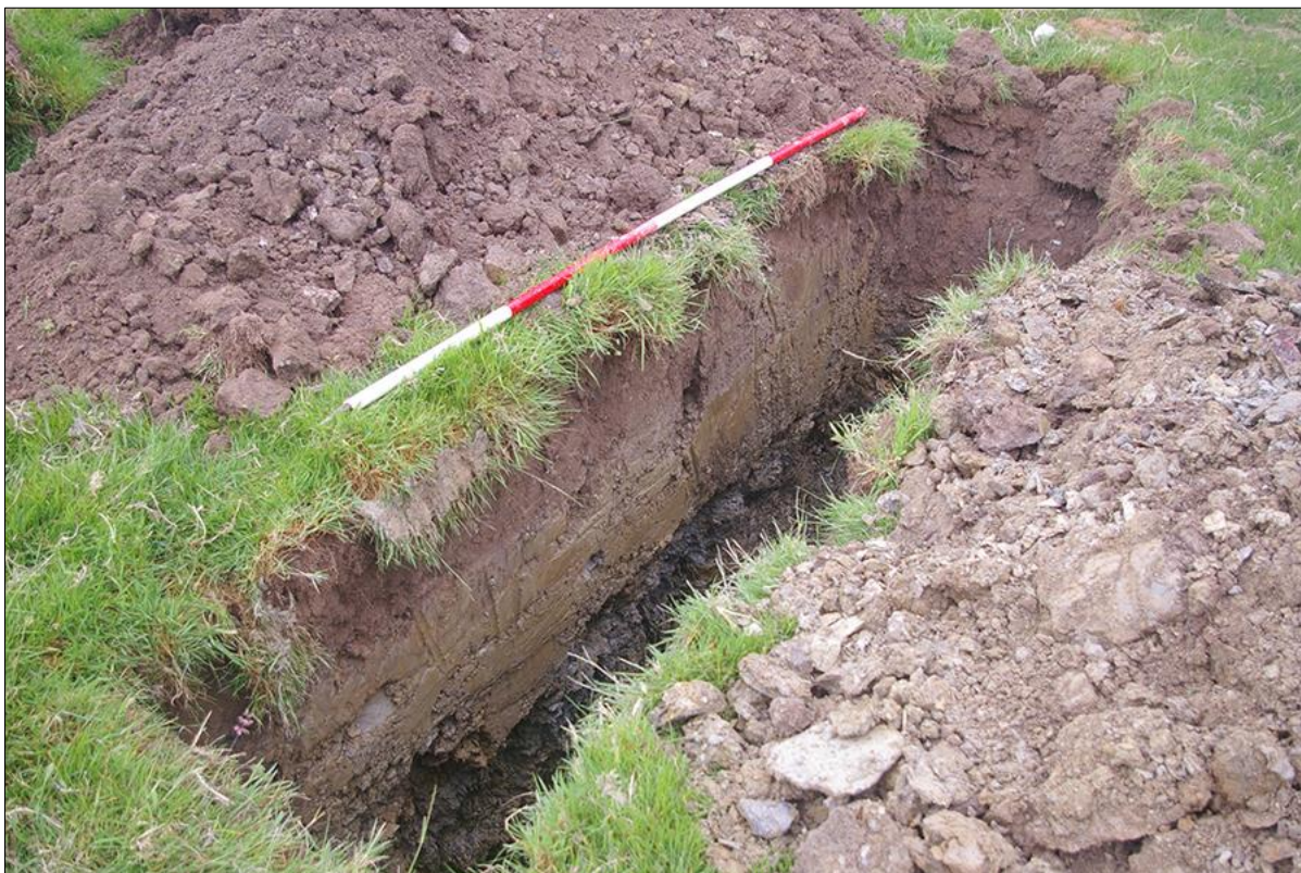
FIGURE 6: TRIAL-PIT 08, NORTH-EAST FACING SECTION DEMONSTRATING ITS DIFFERENT STRATIGRAPHIC MAKE-UP WITH 'DRY' DEPOSITS OVER NATURAL BEDROCK RATHER THAN RIVER GRAVELS; VIEWED FROM THE EAST (2M SCALE).
