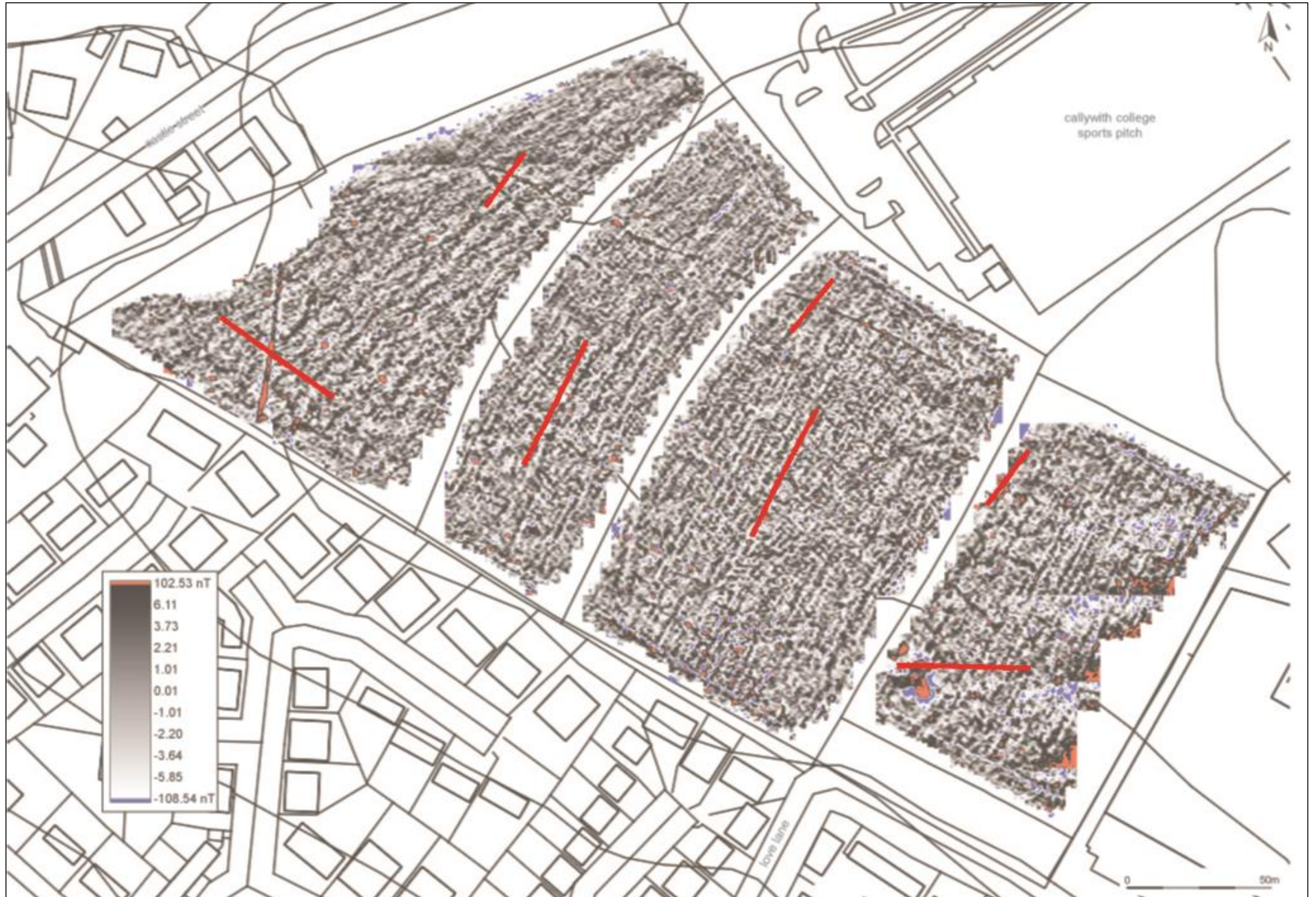
FIGURE 9: SITE PLAN; SHOWING TRENCH LOCATIONS OVERLAYING RED-GREEN-BLUE SHADE PLOT OF GRADIOMETER SURVEY (BAMPTON 2020).
