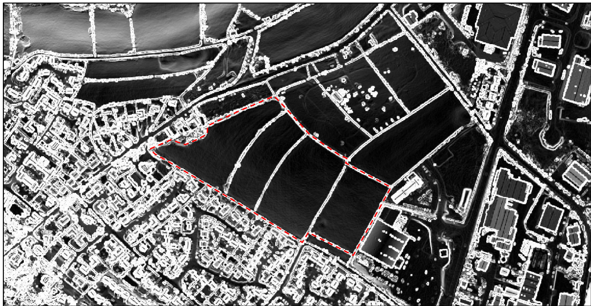
FIGURE 18: IMAGE DERIVED FROM LIDAR DATA; THE SITE IS OUTLINED IN RED (PROCESSED USING QGIS VER2.18.4, TERRAIN ANALYSIS/SLOPE, VERTICAL EXAGGERATION 3.0). DATA: CONTAINS FREELY AVAILABLE DATA SUPPLIED BY NATURAL ENVIRONMENT RESEARCH COUNCIL (CENTRE FOR ECOLOGY & HYDROLOGY; BRITISH ANTARCTIC SURVEY; BRITISH GEOLOGICAL SURVEY); ©NERC.
