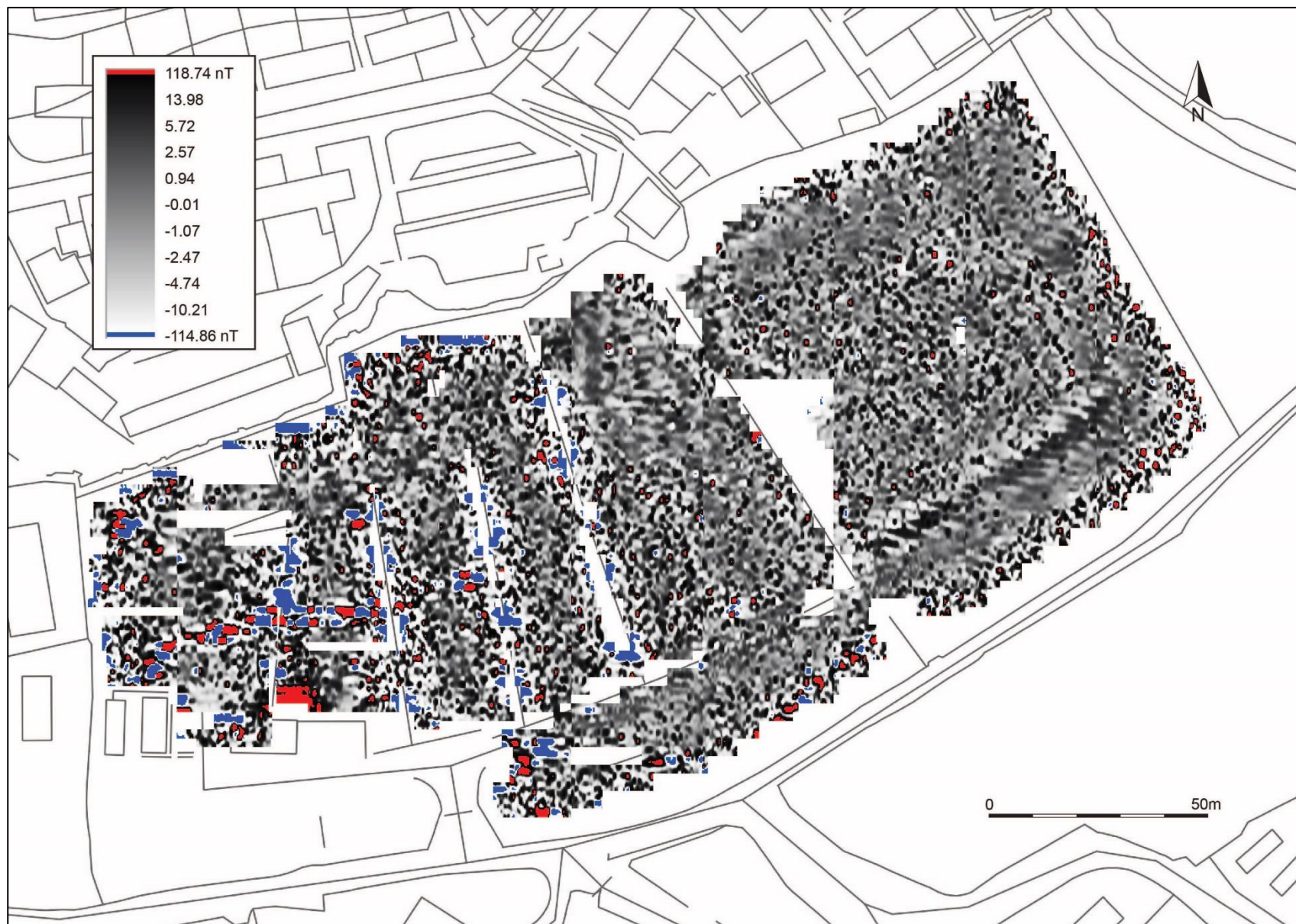
FIGURE 18: RED-GREY-BLUE SHADE PLOT OF GRADIOMETER SURVEY DATA; BAND WEIGHT EQUALISED; GRADIATED SHADING.
