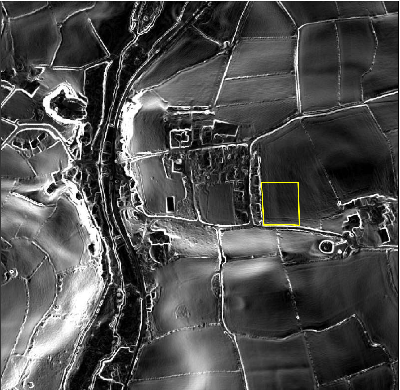
FIGURE 18: TOPOGRAPHICAL IMAGE BASED ON LIDAR DATA. THIS IS A QGIS-GENERATED IMAGE (TERRAIN ANALYSIS>SLOPE) OF TELLUS LIDAR SURVEY DATA [CONTAINS FREELY AVAILABLE LIDAR DATA SUPPLIED BY NATURAL ENVIRONMENT RESEARCH COUNCIL (CENTRE FOR ECOLOGY & HYDROLOGY; BRITISH ANTARCTIC SURVEY; BRITISH GEOLOGICAL SURVEY), ©NERC 2020.
