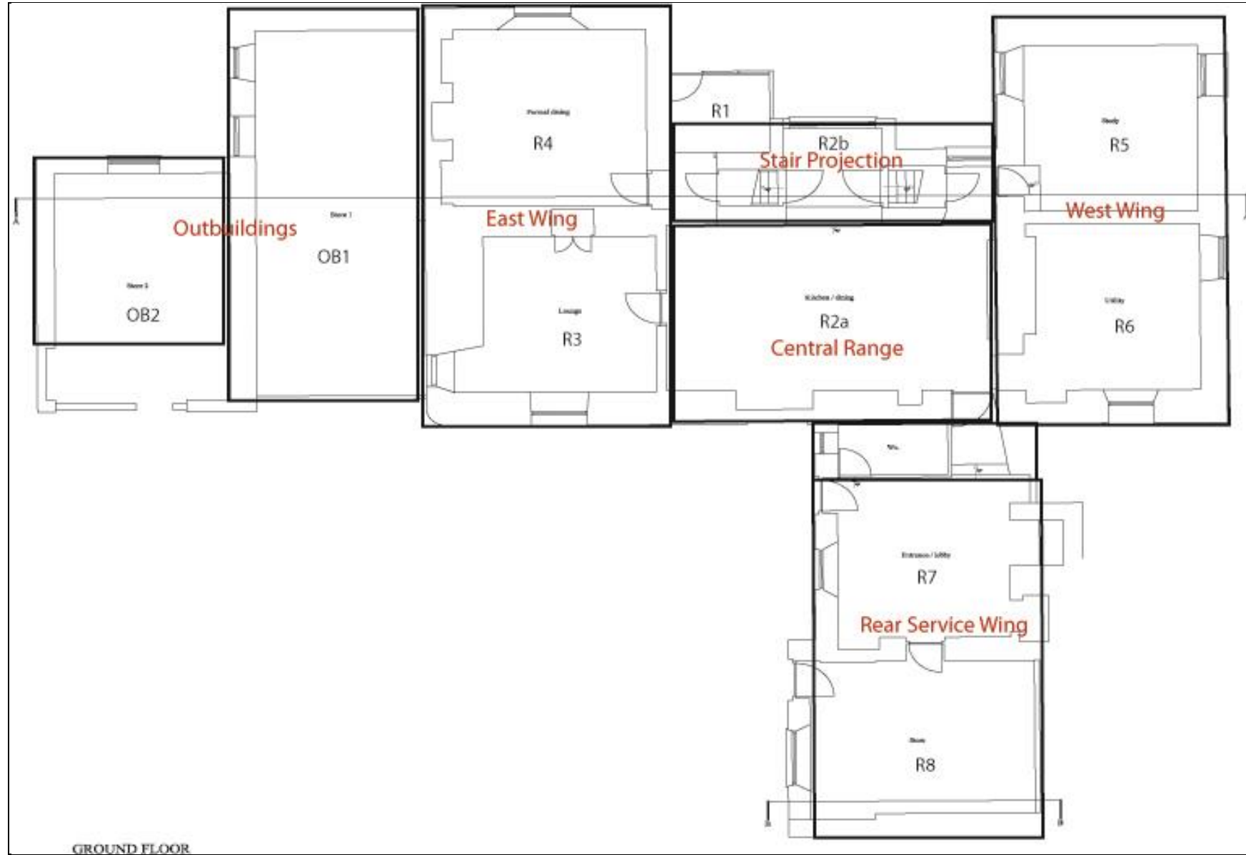
FIGURE 13: PLAN OF THE FARMHOUSE WITH RELATIONSHIP OF BLOCKS (FROM PLANS AS SUPPLIED BY AGENT).
