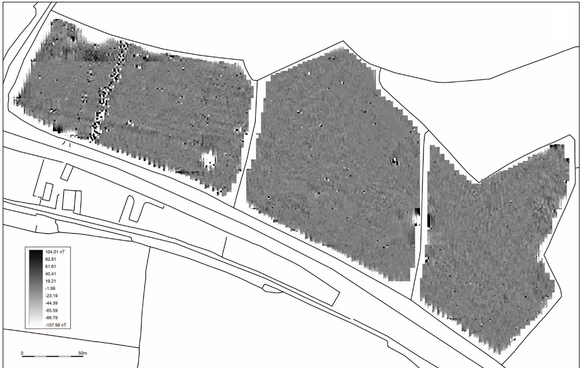
FIGURE 12: SHADE PLOT OF GRADIOMETER SURVEY DATA; BAND WEIGHT EQUALISED; GRADIATED SHADING.
