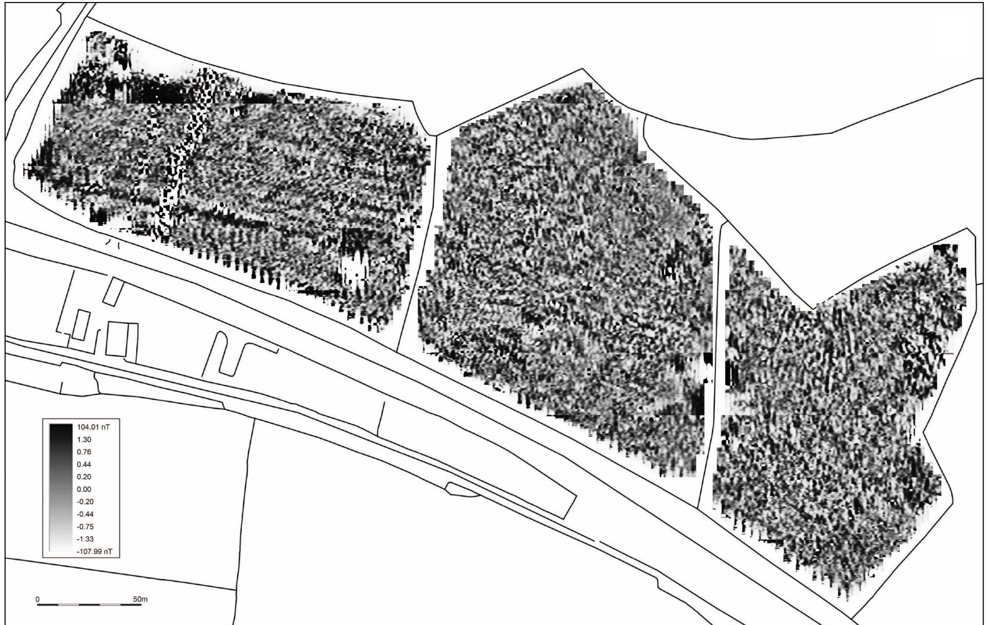
FIGURE 13: SHADE PLOT OF GRADIOMETER SURVEY DATA; BAND WEIGHT EQUALISED; GRADIATED SHADING.
