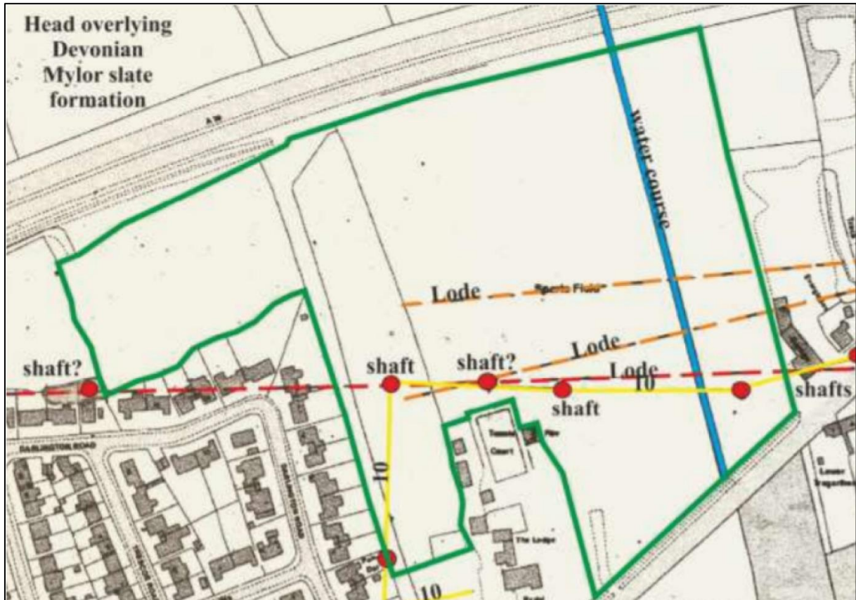
FIGURE 12: COMPOSITE IMAGE SHOWING THE LODES AND PROBABLE SHAFTS ON THE SITE (FROM WM 2018).
