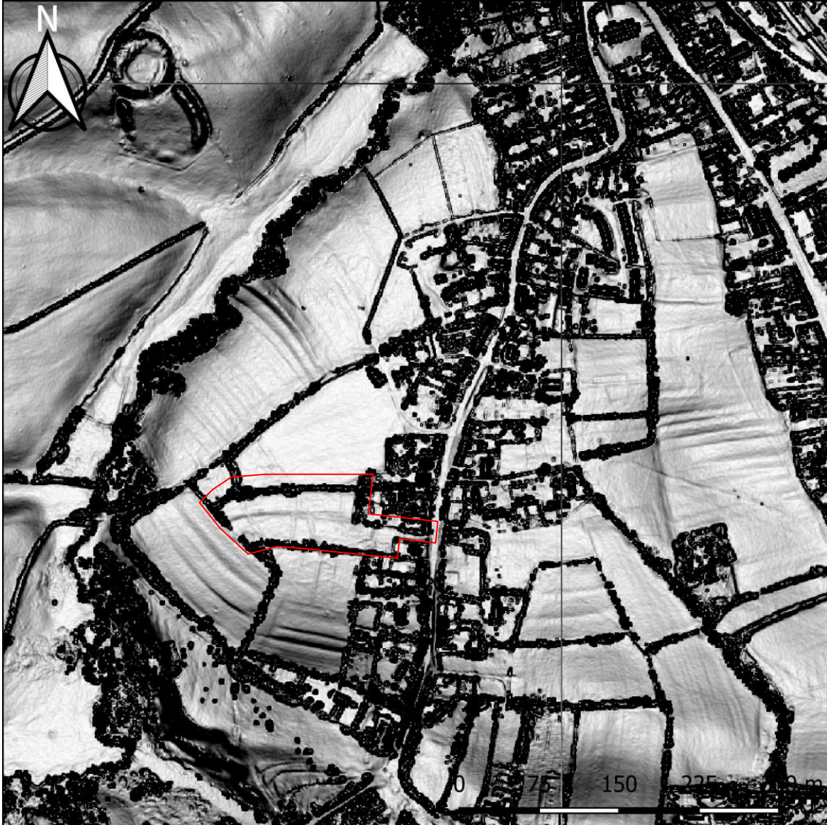
FIGURE 12: IMAGE BASED ON 1M DSM LIDAR DATA (DATA PROCESSED WITH QGIS 3.8, ANALYSIS>SLOPE) (USES ENVIRONMENT AGENCY LIDAR DATA, OPEN GOVERNMENT LICENCE V.3.0 2019); THE SITE IS INDICATED.
