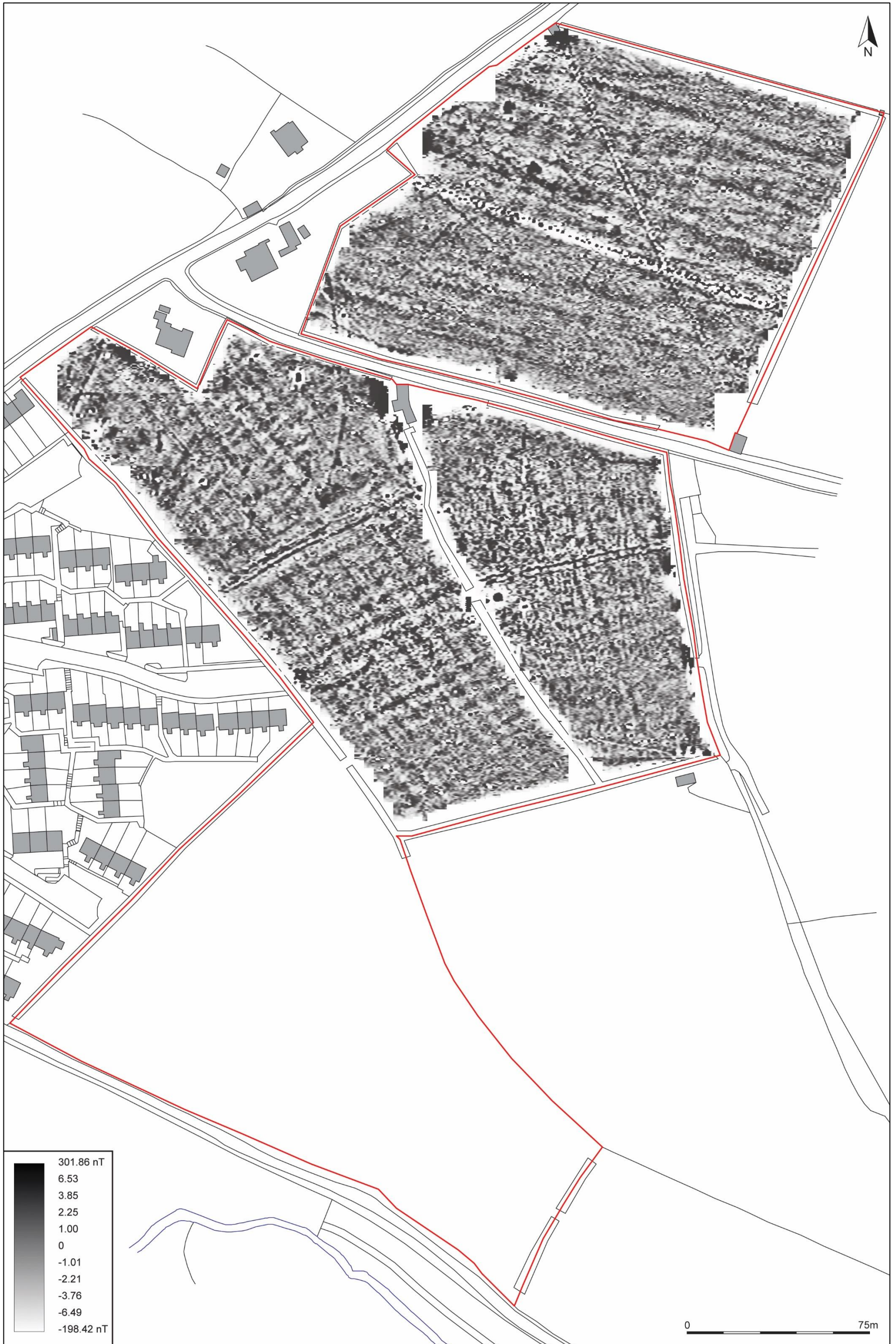
GREYSCALE PLOT OF GRADIOMETER SURVEY DATA; BAND WEIGHT EQUALISED, GRADIATED SHADING.
