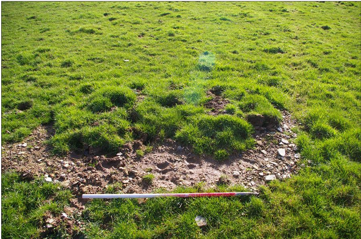
30. DETAIL OF THE BACKFILLED GEOTECHNICAL INVESTIGATION PIT WITHIN F3; VIEWED FROM THE NORTH-WEST (1M SCALE).
