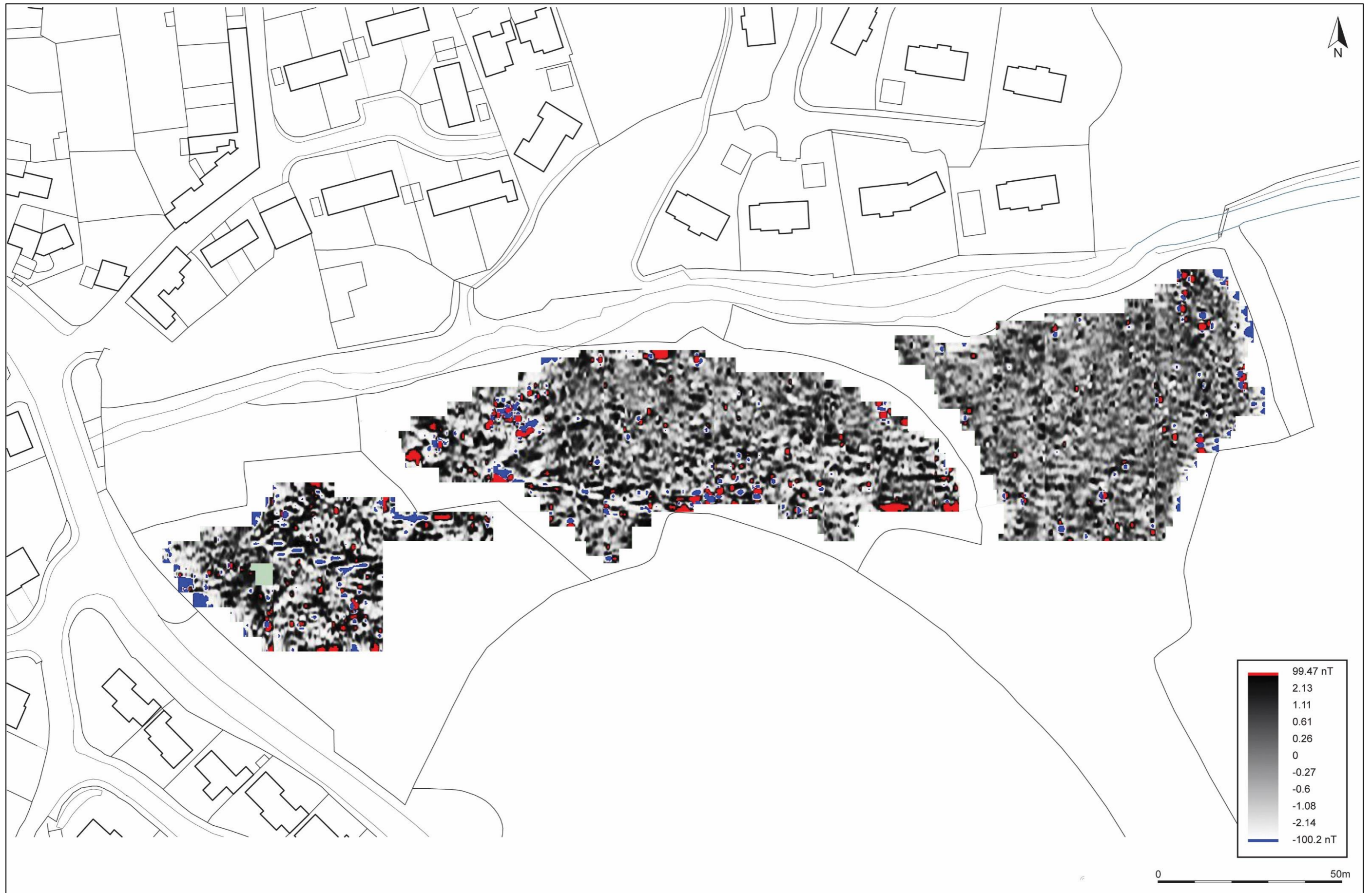
FIGURE 7: RED GREYSCALE BLUE SHADE PLOT OF GRADIOMETER SURVEY DATA; BAND WEIGHT EQUALISED, GRADIATED SHADING.
