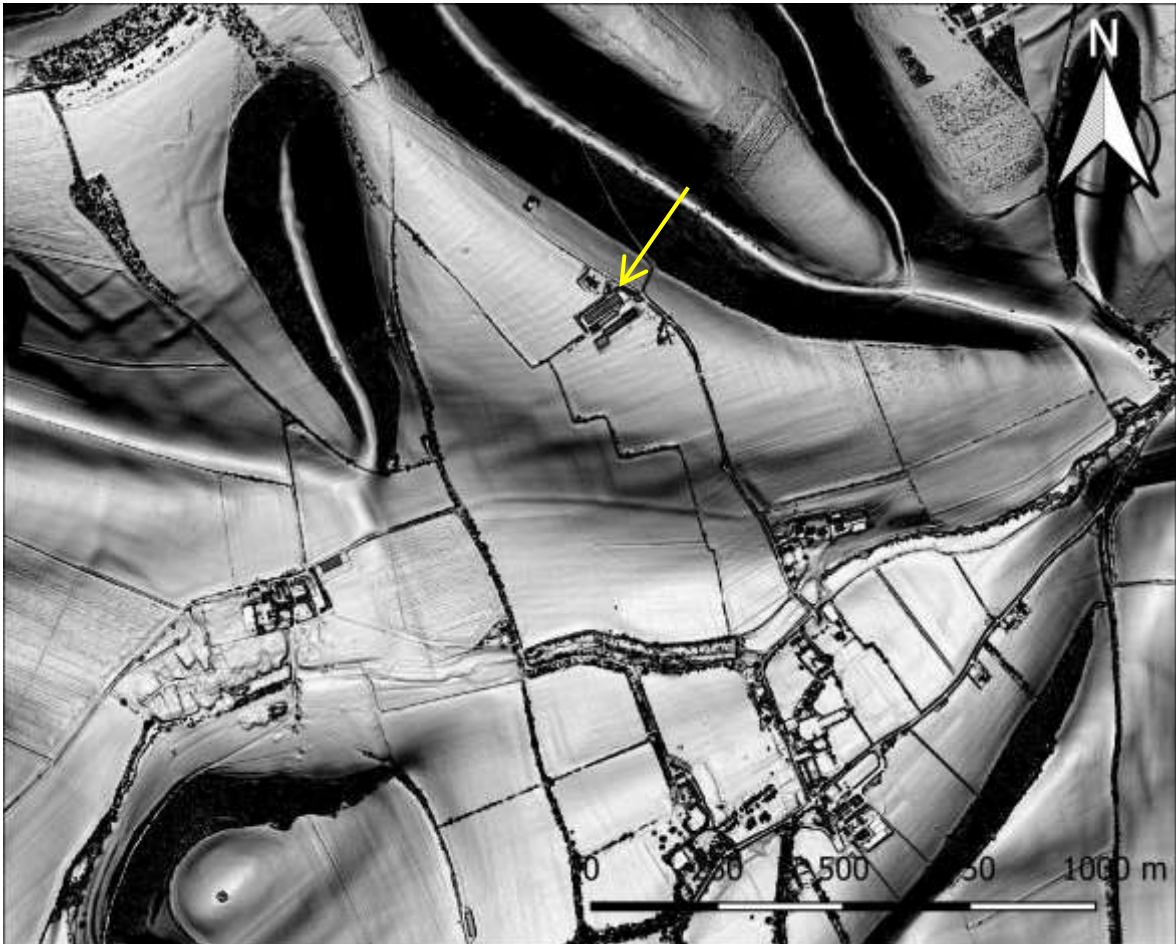
FIGURE 7: IMAGE BASED ON 1M DSM LIDAR DATA (DATA PROCESSED WITH QGIS 3.8, ANALYSIS>SLOPE) (USES ENVIRONMENT AGENCY LIDAR DATA, OPEN GOVERNMENT LICENCE V.3.0 2020); THE LOCATION OF THE MAST IS INDICATED.
