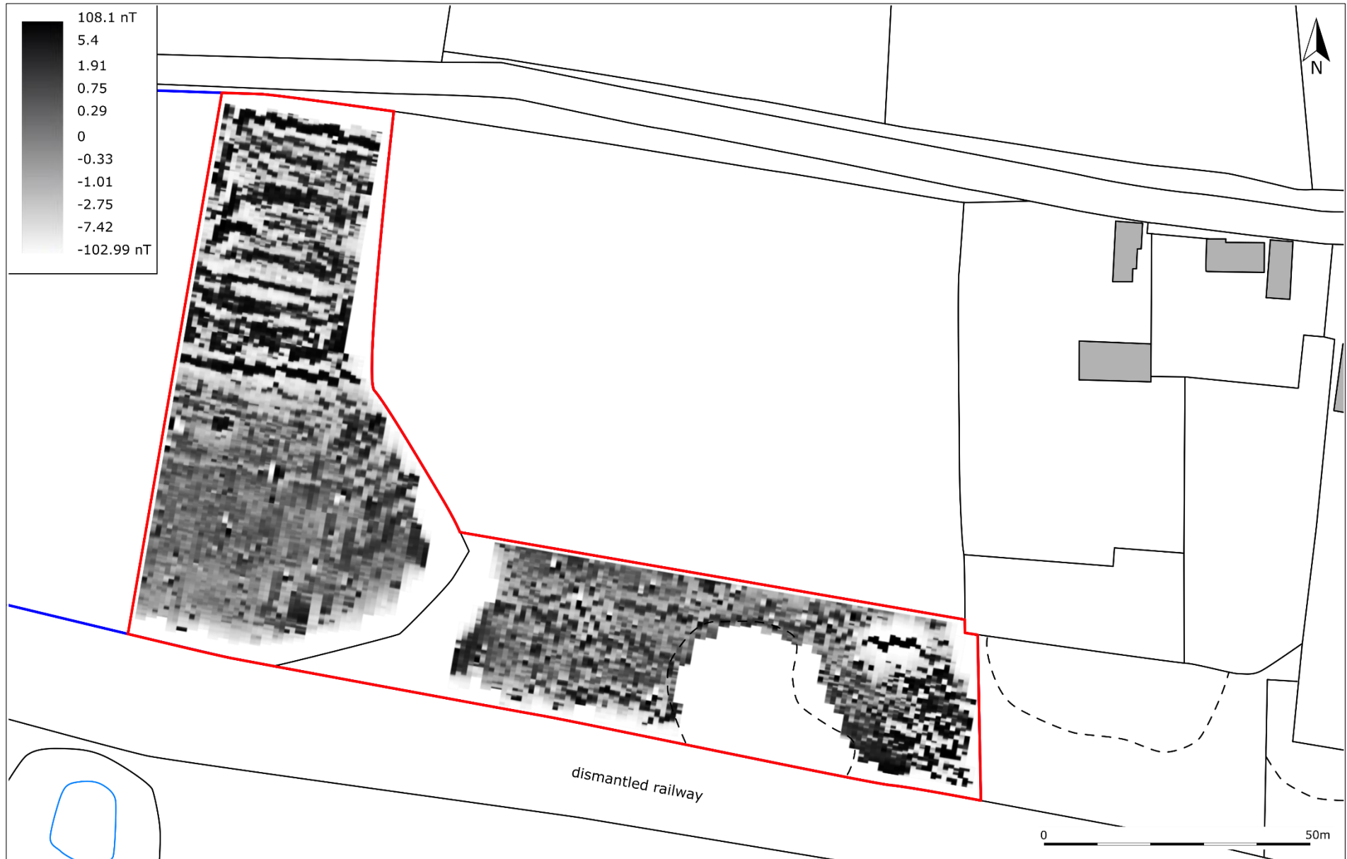
FIGURE 3: SHADE PLOT OF GRADIOMETER SURVEY; MINIMAL PROCESSING.
