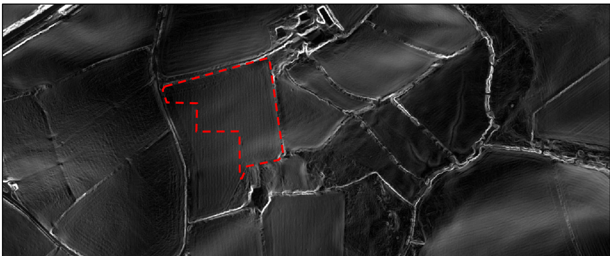
FIGURE 9: IMAGE DERIVED FROM LIDAR DATA; THE SITE IS OUTLINED IN RED (PROCESSED USING QGIS VER2.18.4, TERRAIN ANALYSIS/SLOPE, VERTICAL EXAGGERATION 3.0). DATA: CONTAINS FREELY AVAILABLE DATA SUPPLIED BY NATURAL ENVIRONMENT RESEARCH COUNCIL (CENTRE FOR ECOLOGY & HYDROLOGY; BRITISH ANTARCTIC SURVEY; BRITISH GEOLOGICAL SURVEY); ©NERC.
