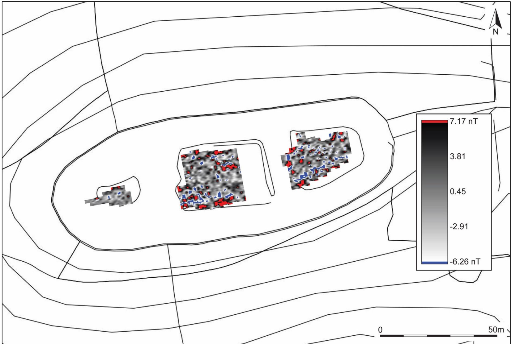
FIGURE 8: RED-GREY-BLUE SHADE PLOT OF MAGNETOMETRY SURVEY DATA; GRADIATED SHADING; CLIPPED BY 1SD (STANDARD DEVIATION).
