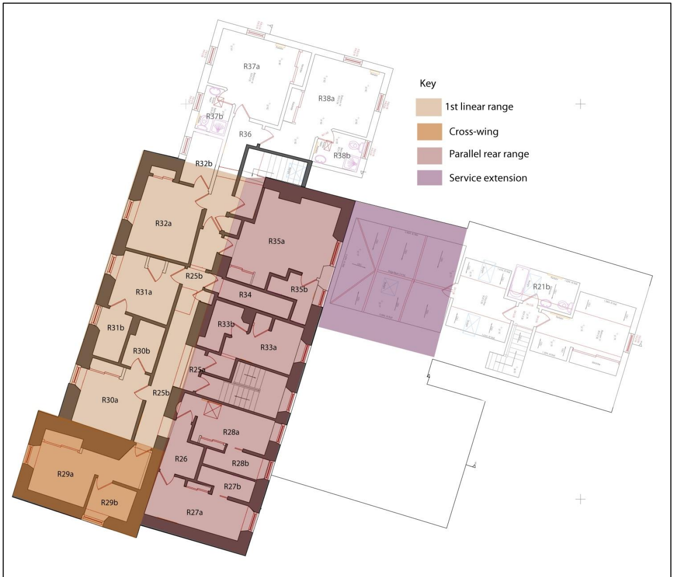
FIGURE 20: PHASED PLAN OF FIRST FLOOR OF TREVANION HOUSE (PLANS SUPPLIED BY AGENT).
