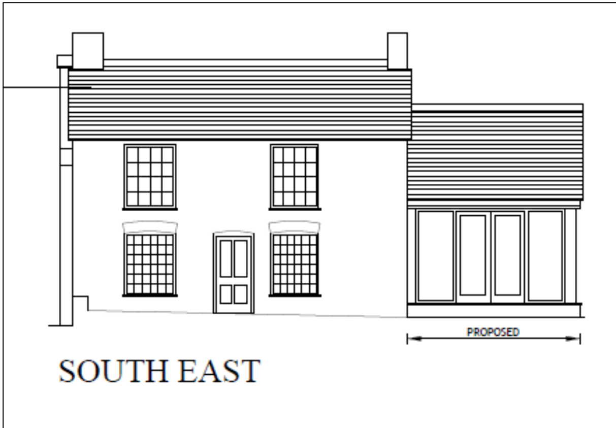
THE PROPOSED DRAWINGS OF THE EAST GABLE OF THE PROPOSED EXTENSION; AS SUPPLIED BY AGENT.
